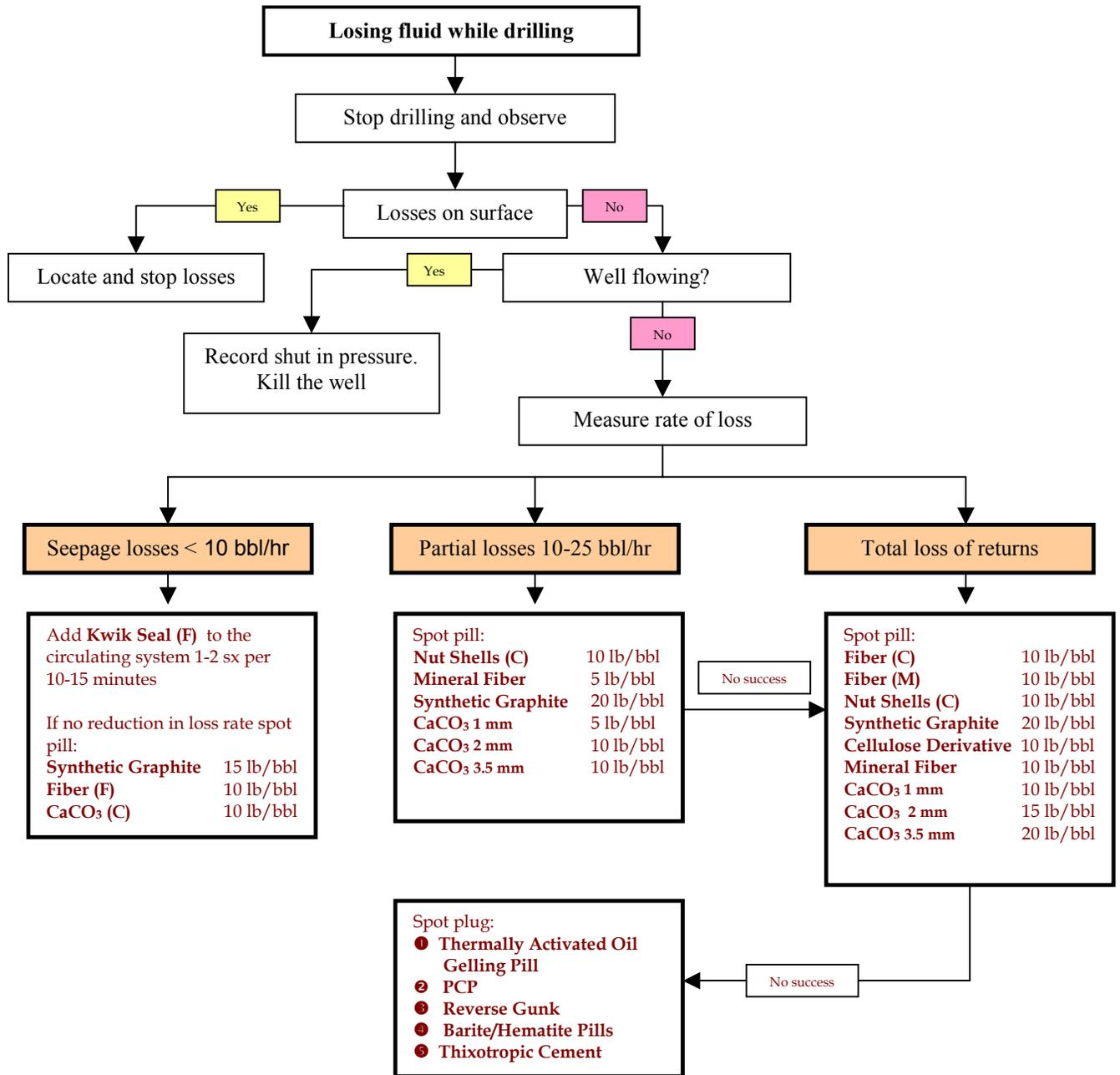
Fig. 4: The Lost Circulation Assessment and Planning decision tree covering conventional, specialized and contingency lost circulation treatments for a naturally fractured carbonate well in Central Asia.
