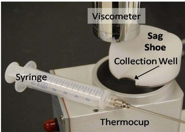
Figure 4: Basic equipment for VSST method (digital balance not shown).
