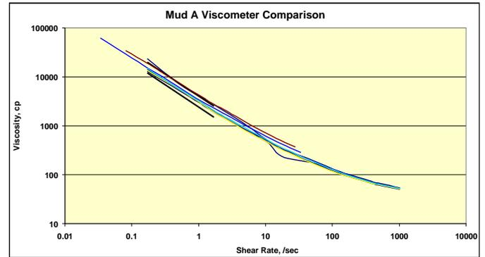
Figure 9: Comparison of Drilling Fluid A data for all three viscometers at all labs
