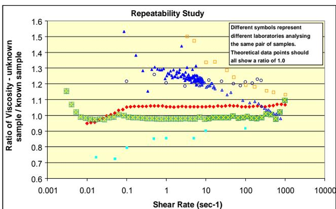
Figure 5: Repeatability of viscosity measurements on drilling fluid samples in a previous sag study.<sup>11</sup>
