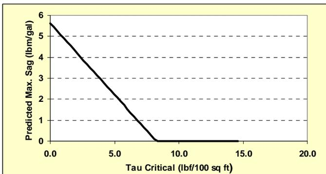
Figure 7: Wall shear stress vs. maximum measured dynamic barite sag.<sup>14</sup>
