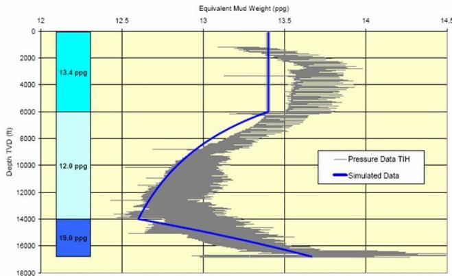
Figure 2: Downhole density changes measured while running the drillstring in the hole.<sup>4</sup>
