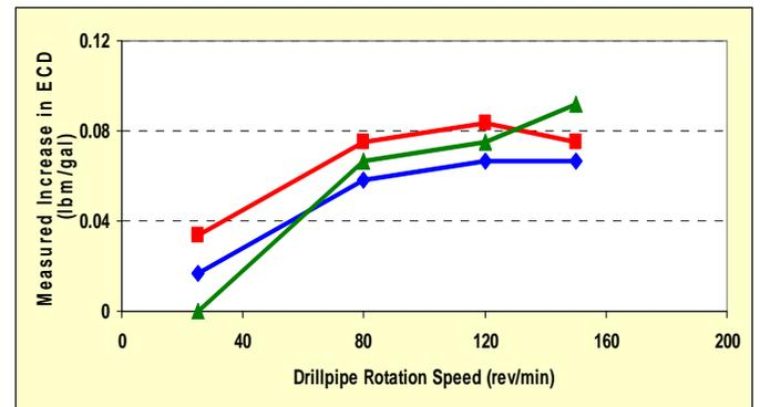
Figure 3: North Sea fingerprinting exercises for three flow rate and drillstring rotation speed combinations.<sup>6</sup>
