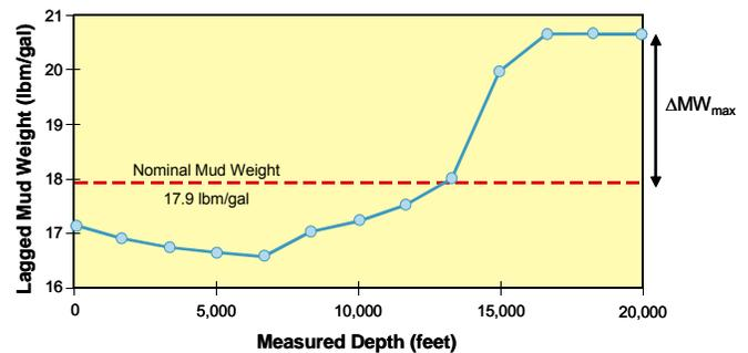
Figure 1: Example surface density profile based on bottoms-up data.
