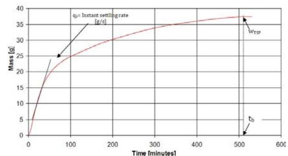
Figure 12: Example output from the direct weight method.
