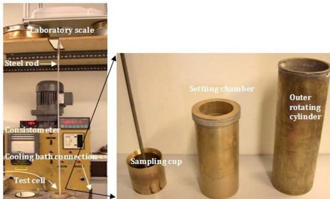
Figure 10: Photograph of direct weight-monitoring equipment
