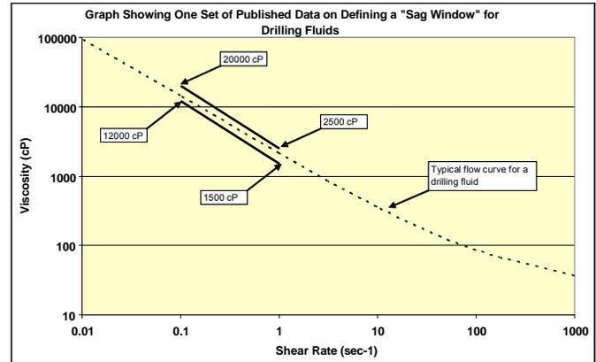
Figure 6 – “Sag Window” for drilling fluids vs shear rate.<sup>13</sup>
