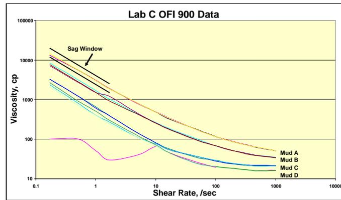
Figure 8: Comparison of rheology data for multiple runs of four drilling fluids within one lab (three runs per drilling fluid).
