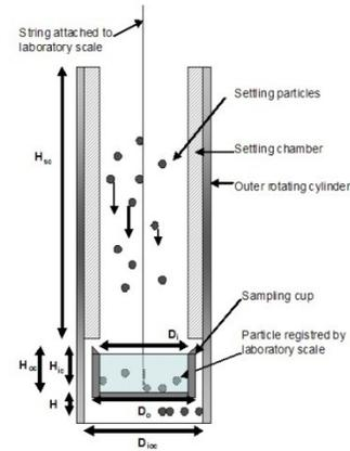
Figure 11: Schematic of direct weight-monitoring equipment.
