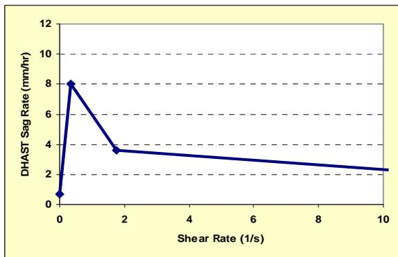
Figure 14: DHAST Sag Rate vs. Shear Rate for a North Sea production well.<sup>16</sup>
