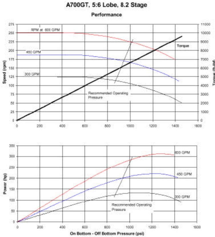
Fig. 4- Power Curve for the A700GT5:6 motor
