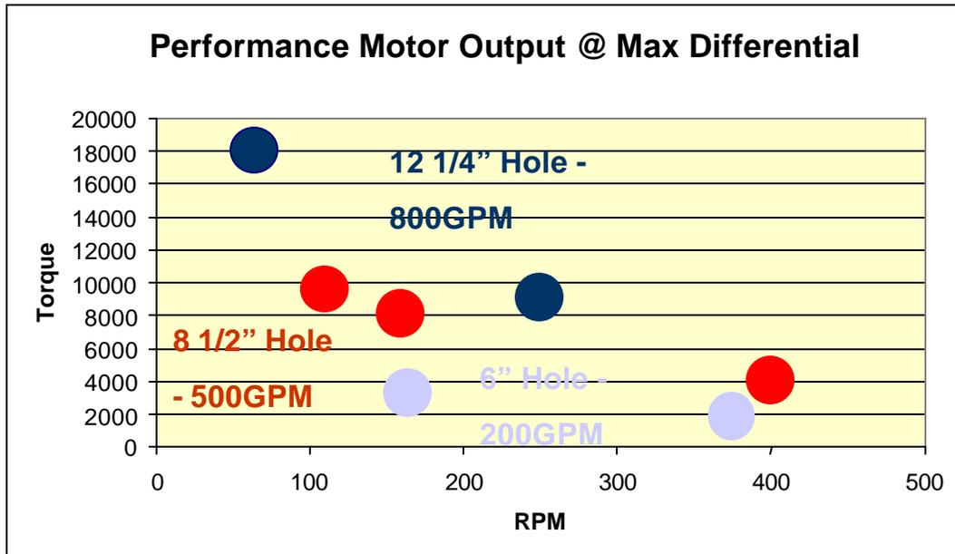
Fig. 2- Performance motor output.
