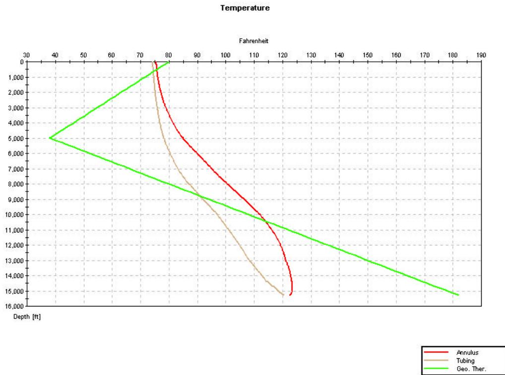
Figure 2A. Dynamic temperature profile of deepwater well
