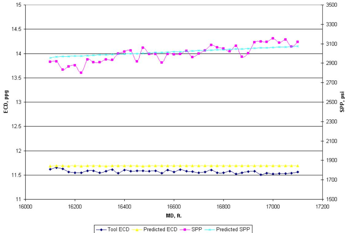
Figure 7. Predicted vs Measured Pressures in 12 1/4" Section – Case History #1
