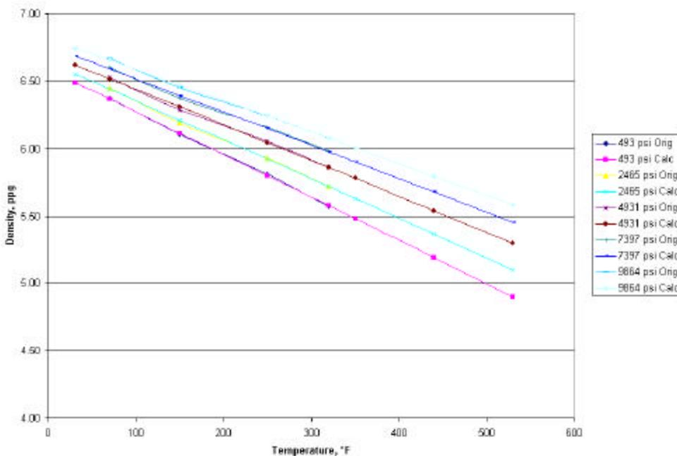
Figure 5. PVT on synthetic base fluid (Isobar)
