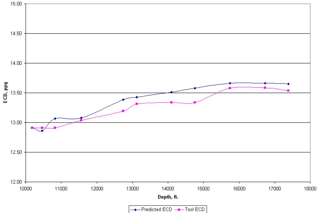
Figure 12. ECD's Without Theoretical Cuttings Bed
