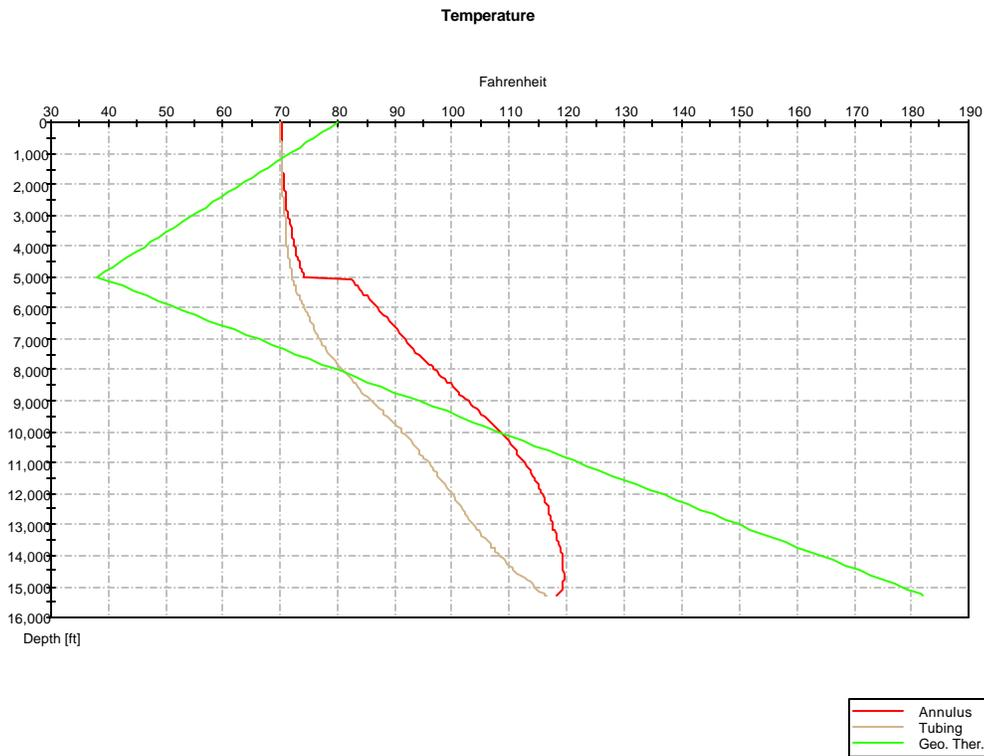
Figure 2B. Dynamic temperature profile of deepwater well with booster pump
