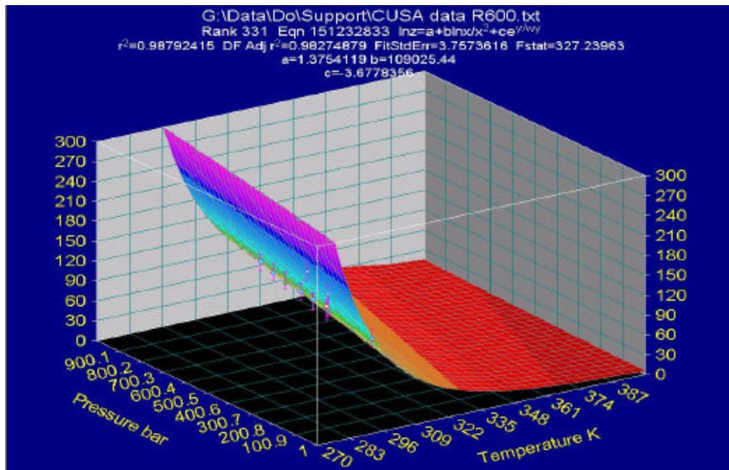
Fig. 3- 3-Dimensional curve Fit of HT-HP rheological data.
