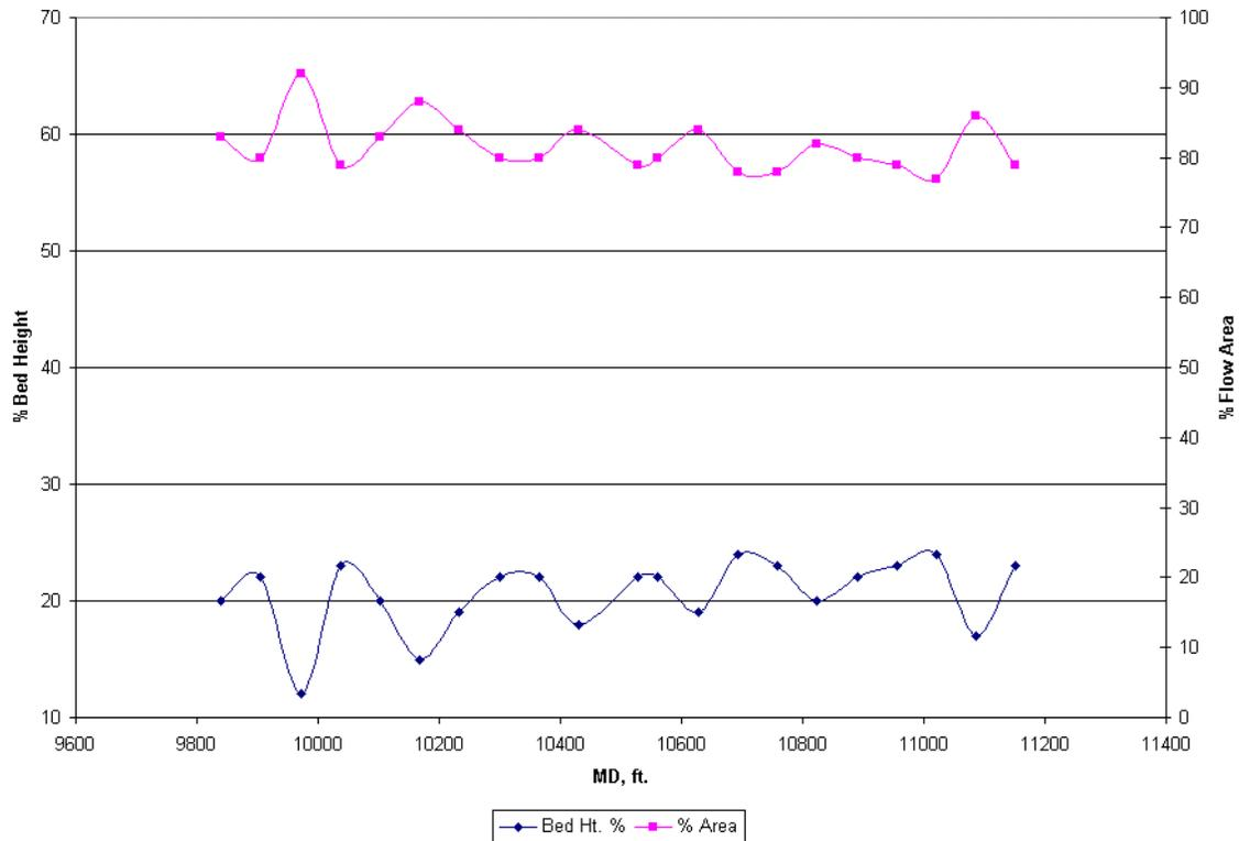
Figure 11. Theoretical Bed Height/Annular Flow Area Reduction
