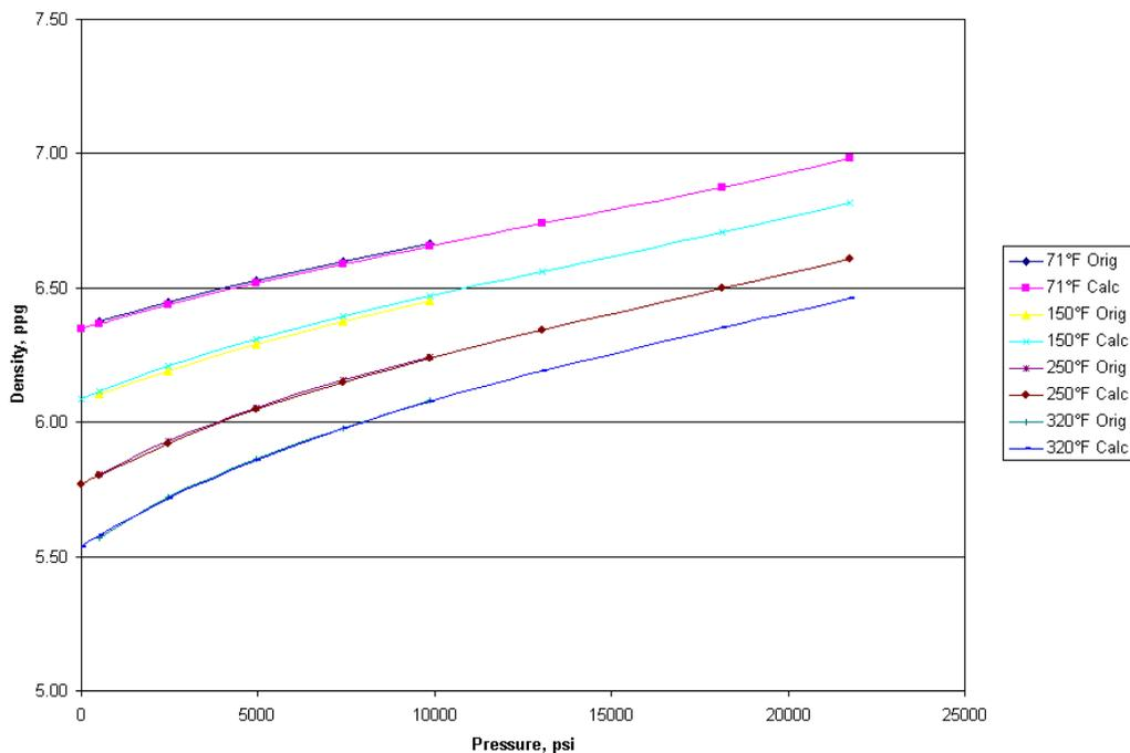
Figure 4. PVT on synthetic base fluid (Isotherm)
