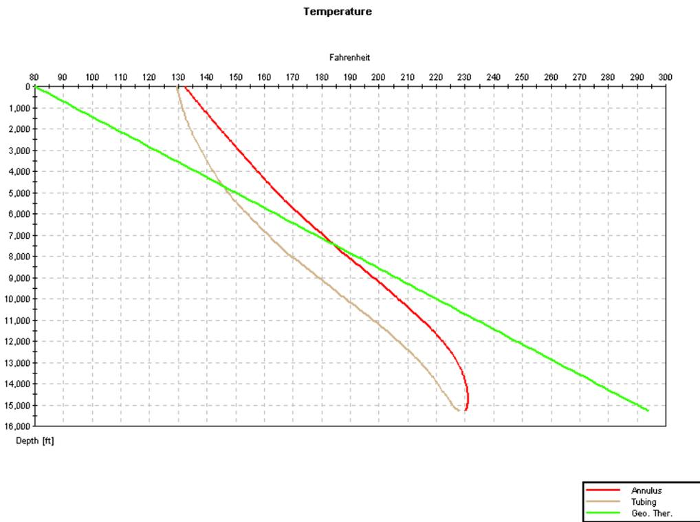
Figure 1. Dynamic temperature profile of land well
