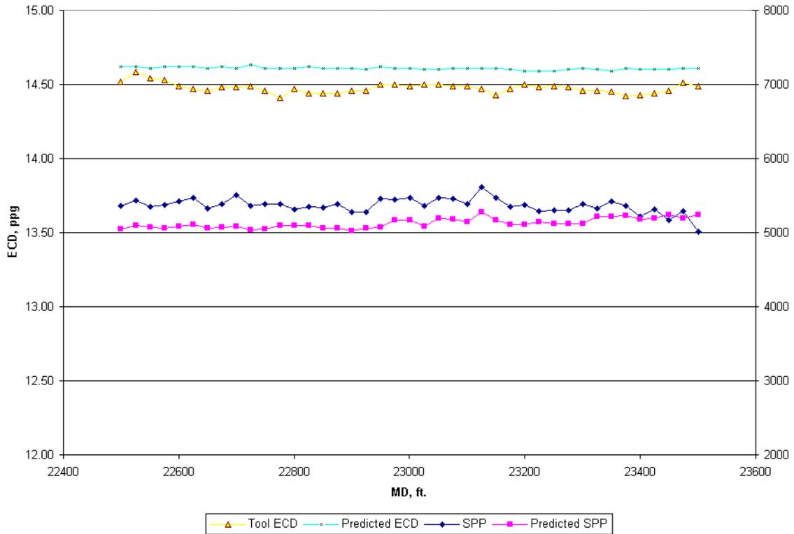
Figure 9. Predicted vs Actual Pressures in 11.4” Section – Case History #2
