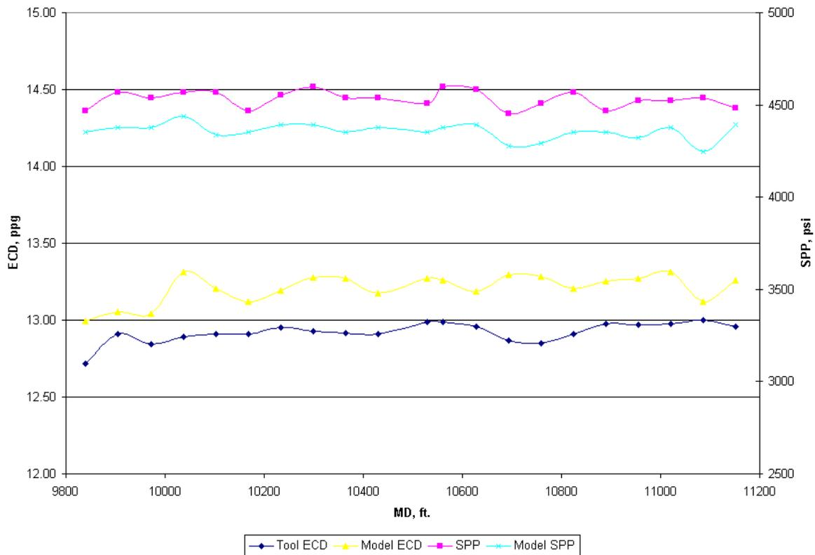
Figure 10. Predicted vs. Actual Pressures in 12 ¼” Section- Case History #3 – poor hole cleaning.
