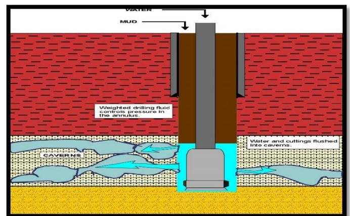
Figure 7. Floating Mud Cap Drilling Method (Baker Hughes, 1999<sup>6</sup>)
