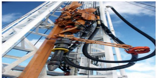
Figure 5. Top Drive and Casing Drive (Tessari et al., 2006 <sup>10</sup>)
