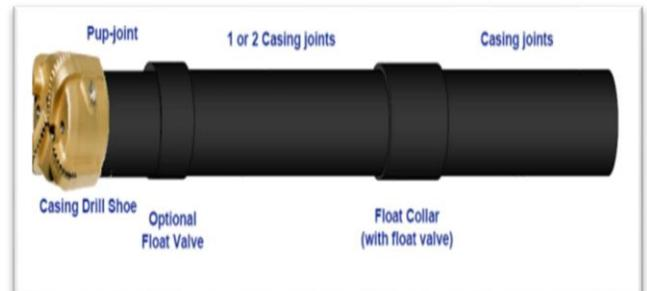
Figure 4. BHA of CWD Assembly (Gallardo et al., 2010 <sup>9</sup>)
