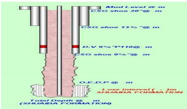
Figure 6. Lost Circulation Mud in the Shuaiba Formation
