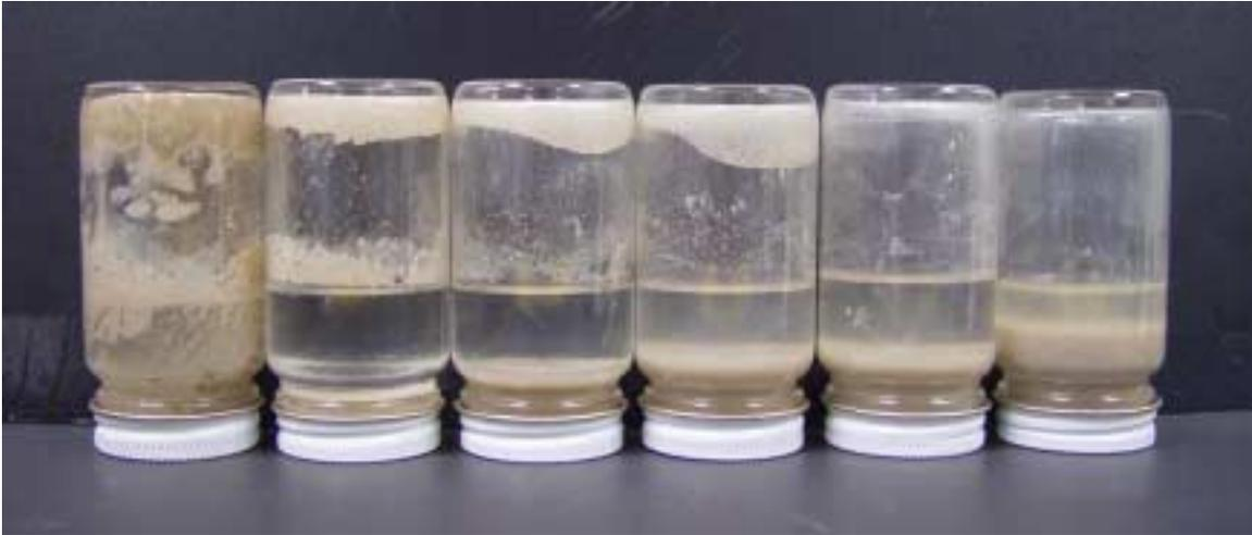
**Figure 4. Cleaner Capacity Test.** Using 5 grams of mud/sand mixture in each bottle, 30 mL of wash solution is applied with increasing surfactant concentration. From left to right, 1,2,3,4,5, 7.5 and 10 vol% surfactant is applied. 1% is not able to clean the mud off the glass. At 2,3,4, 5%, synthetic-wet sand remains. By 7.5% concentration, clean glass and no synthetic-wet sand remain. The 5% is marginally clean, 7.5 and higher are clean.
