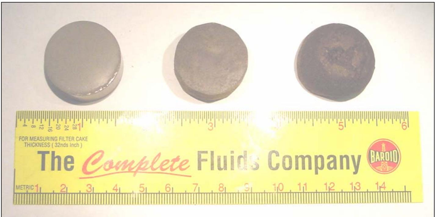
**Fig. 1 - Shale inhibition (Hot Roll/Dispersion) test comparing an SBM with a One-Sack HPWBM**
