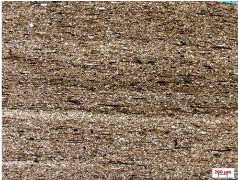
Figure 4 – Section MSF1 (7535.80 – 7536 ft). Fissile clay shale. Note extreme parallelism of clay minerals, fine lamination, and marked predominance of clay-sized materials.
