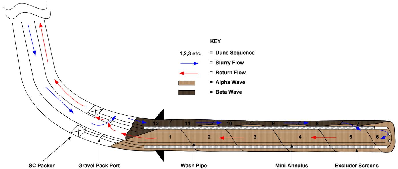
Fig. 4 - Alpha and Beta Wave progression during a horizontal gravel pack.
