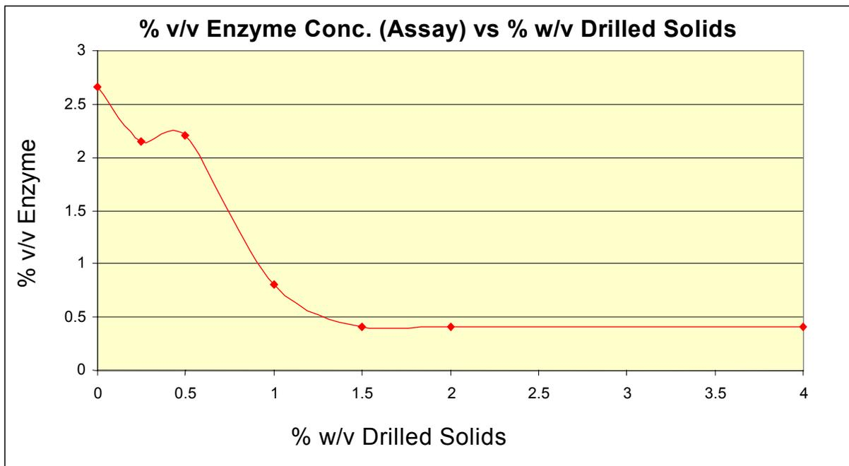
Fig. 7 – Study into the effects of drilled solids on enzyme filtration.
