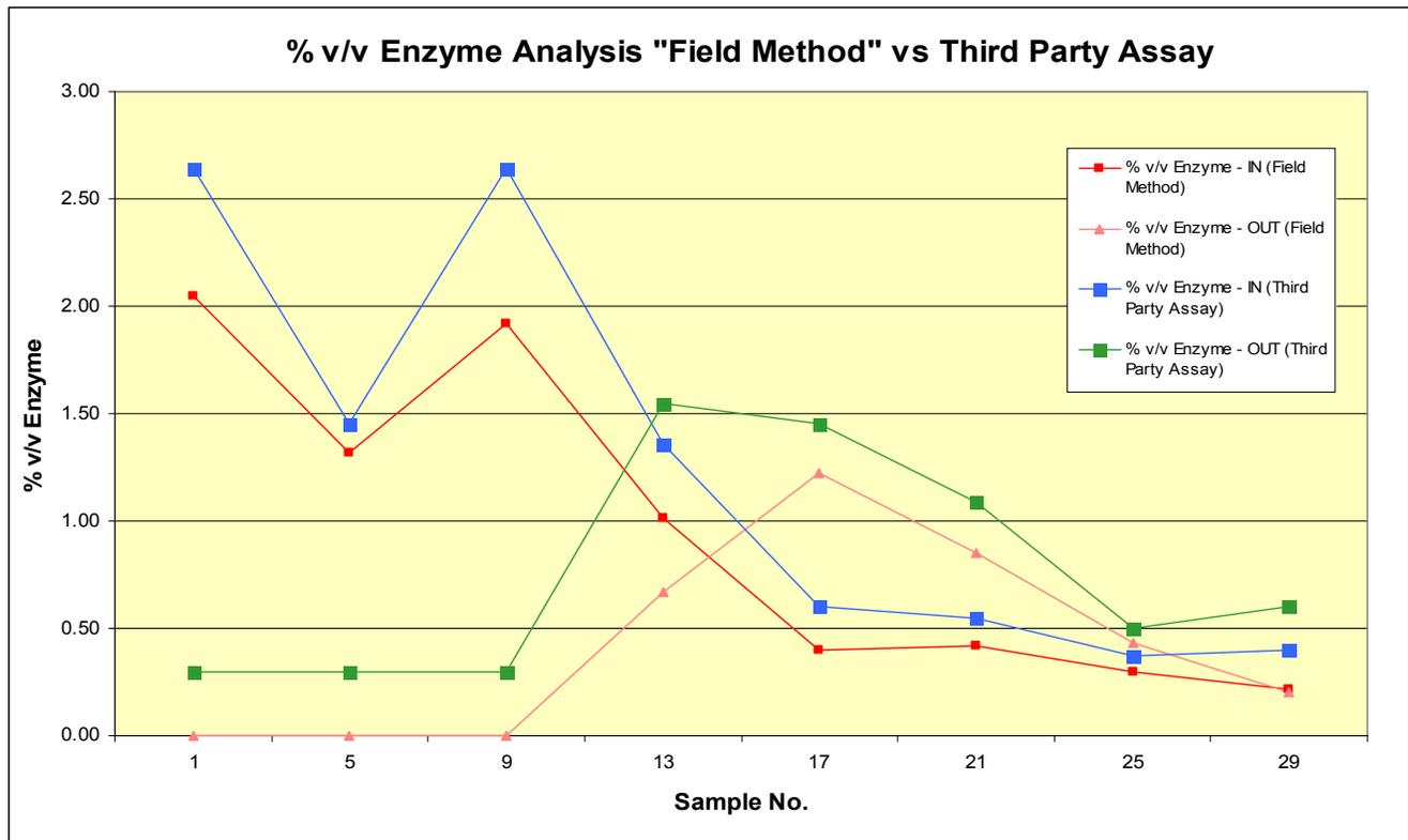
Fig. 5 – Enzyme analysis of suction pit (IN) and return pit (OUT) by “field” method and third-party assay.
