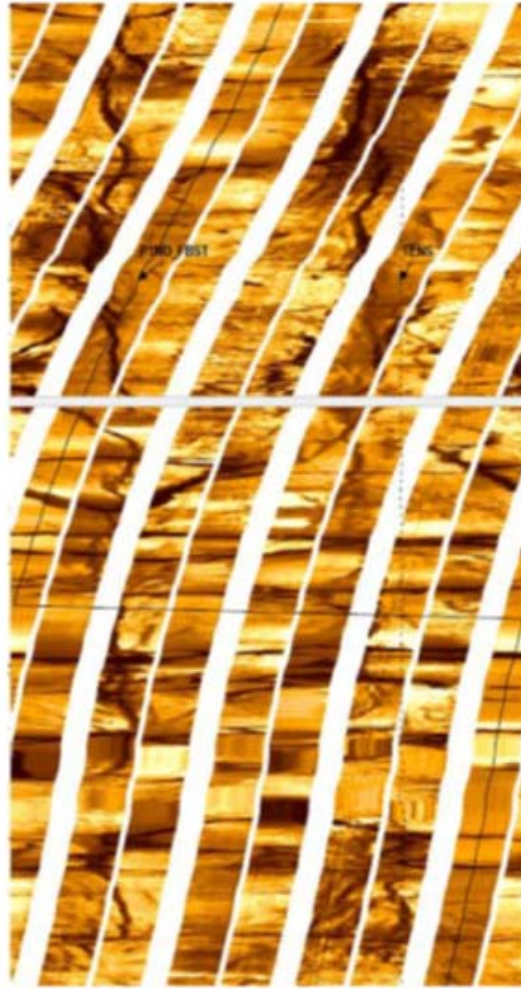
Figure 7 – Selected image of an FMI log from Well 11, 8 3 / 8 -inch wellbore, as processed after controlling losses. Note the fracture patterns which most likely provided the preferential path for losses (Bijjani et al. 2018a)
