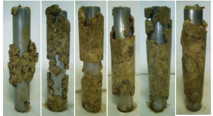
Figure 3 – Accretion profiles for Arne Clay (5-, 10-, 20-, 40-, 60-, and 80-min time intervals).
