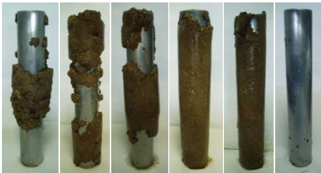
Figure 6 – Accretion profiles for London Clay (5-, 10-, 20-, 40-, 60-, and 80-min time intervals).
