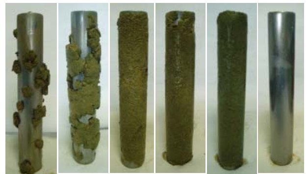
Figure 5 – Accretion profiles for Green-Lillebaelt Clay (5-, 10-, 20-, 40-, 60-, and 80-min time intervals).
