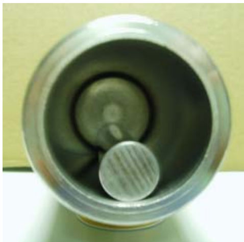
Figure 1 – Accretion Test Cell – Solid Steel Bar (SSB).
