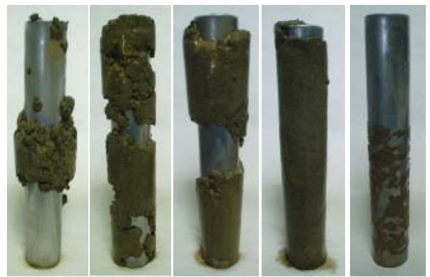
Figure 4 – Accretion profiles for Foss Eikeland Clay (5-, 10-, 20-, 40-, and 60-min time intervals).
