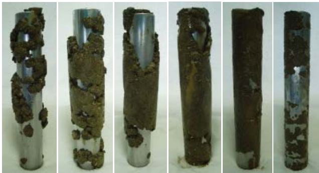
Figure 7 – Accretion profiles for Oxford Clay (5, 10, 20, 40, 60 and 80 minute time intervals).
