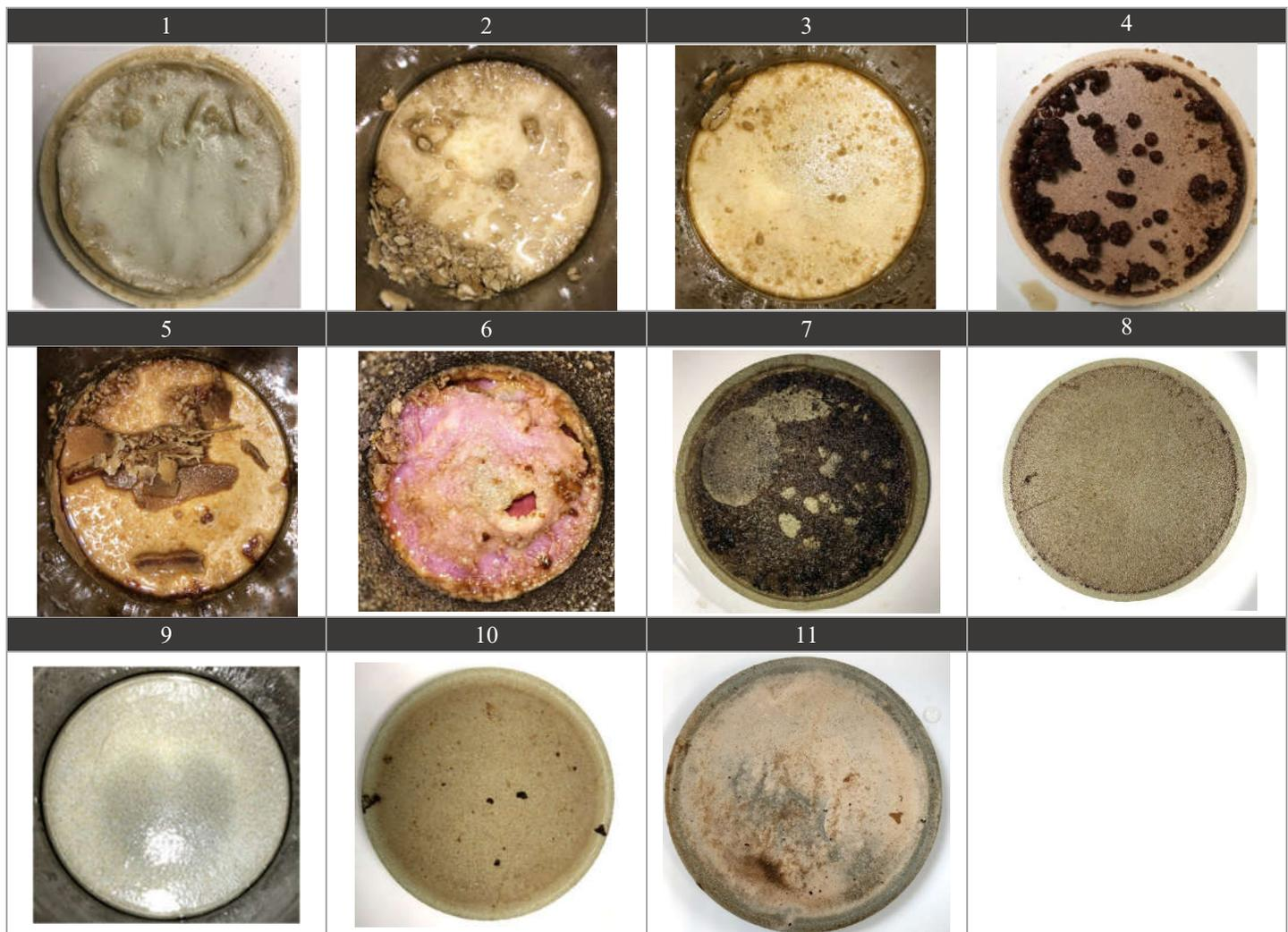
Figure 3 Photos of Simulated Formation Discs after Exposure to HT Acid Precursor Breaker
