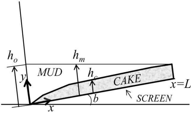
Figure 2. Diagram of the cake section showing the  $x$  and  $y$  coordinate origin and directions with the screen at angle  $\beta$  relative to the horizon. The free surface of the mud is height  $h_m$  above the screen and is a function of position  $x$ . The height of the top surface of the cake,  $h_c$ , is also a function of position  $x$ . The mud height at  $x=0$  is  $h_o$ . The screen length where  $h_m = h_c$  is  $x = L$ .
