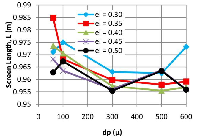
Figure 5: Effect of particle size and porosity on the screen length of the cake section,  $L$ . (Note:  $\epsilon l = \epsilon^L$ ). The tilt angle is 3 degrees.
