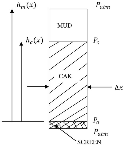
Figure 3: A random slice of the cake section of thickness  $\Delta x$ .
