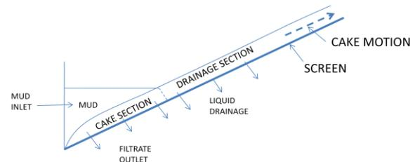
Figure 1: Diagram of the vibrating screen process. The mud with coarse particles enters from the left. A cake of particles forms on the surface of the screen and moves to the right due to the screen vibrations. When the cake moves out of the liquid mud the process becomes one of liquid drainage from the cake. Different phenomena occur in each section requiring different mechanistic models.
