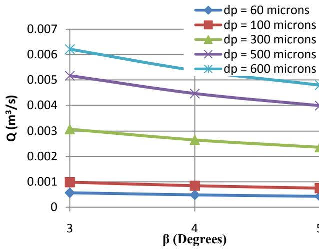
Figure 6: Effect of the tilt angle on volumetric flow rate ( $\text{m}^3/\text{s}$  per meter width of screen) of mud through the screen in the cake section for different particle sizes. The porosity is 0.5.
