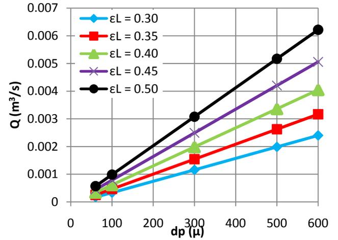
Figure 4: Effect of particle size and porosity on volumetric flow rate (m<sup>3</sup>/s per meter width of screen) through the screen in the cake section. (Note:  $\epsilon l = \epsilon^L$ ). The tilt angle is 3 degrees.
