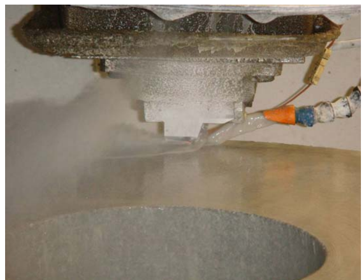
Fig. 1 – VTL cutting granite with single PDC cutter and drilling fluid coolant.
