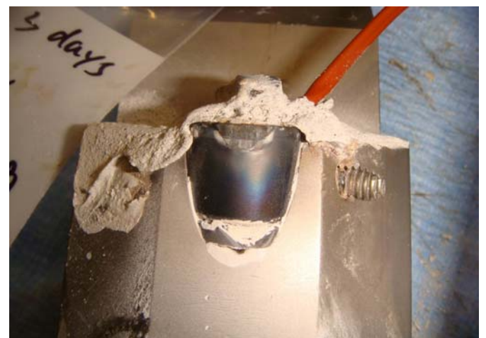
Fig. 7 – Severely worn cutter with shroud of dried cuttings.
