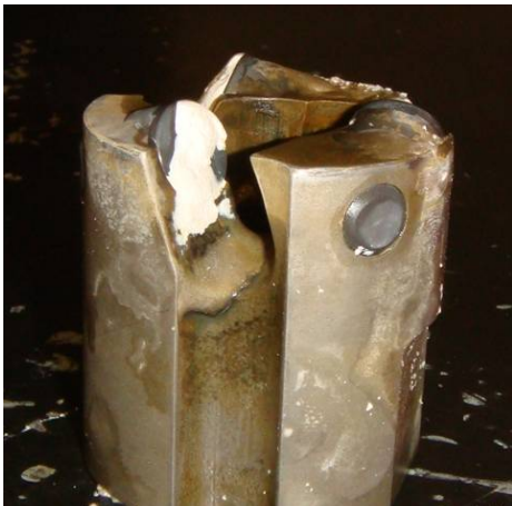
Fig. 5 – Three-cutter core barrel used to cut core in Carthage marble.
