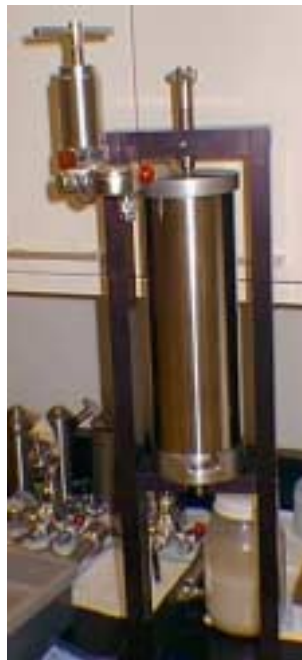
Fig. 3 – Constant-pressure production screen plugging equipment.
