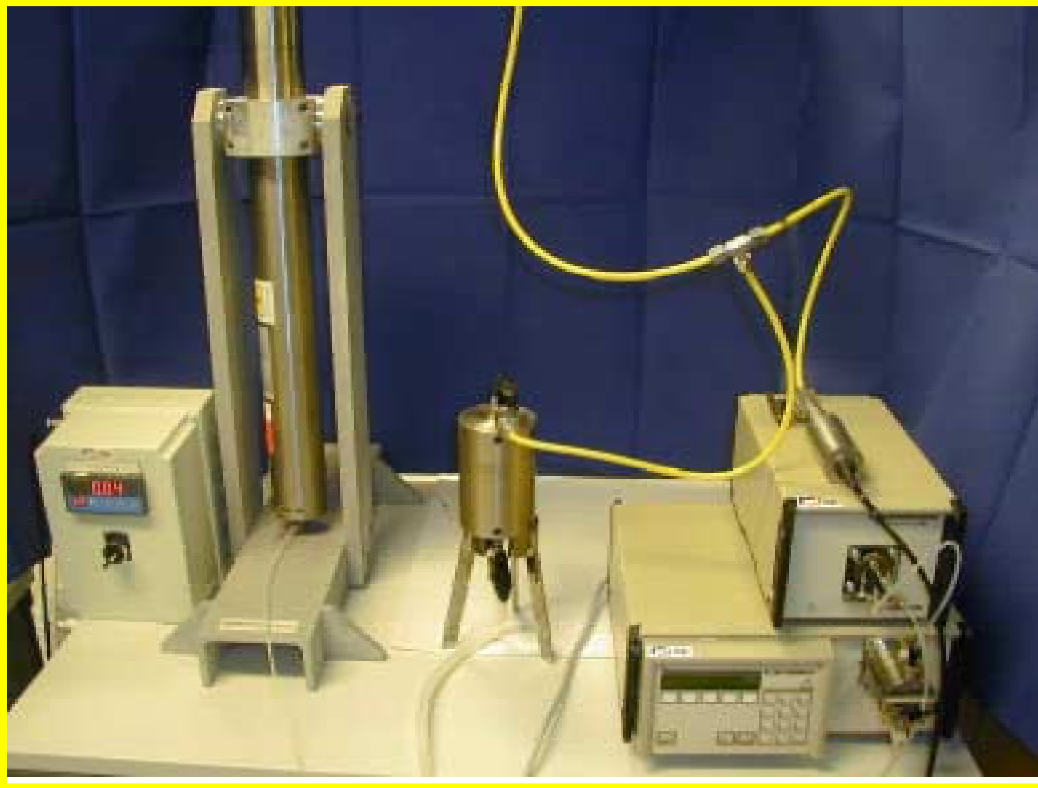
Fig. 2 – Constant-rate laboratory production screen plugging equipment.
