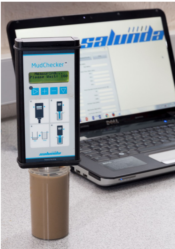
Figure 1 - MudChecker performing a measurement on an oil-based mud sample. Approximately 250ml of mud is needed for each full test (including the salinity measurement), but only 20ml of the mud is consumed in the test.
