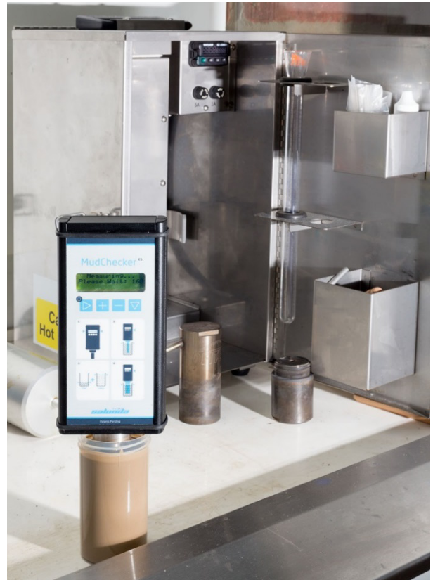
Figure 2: MudChecker requires much less space than the apparatus required for a retort and chemical titration measurement.
