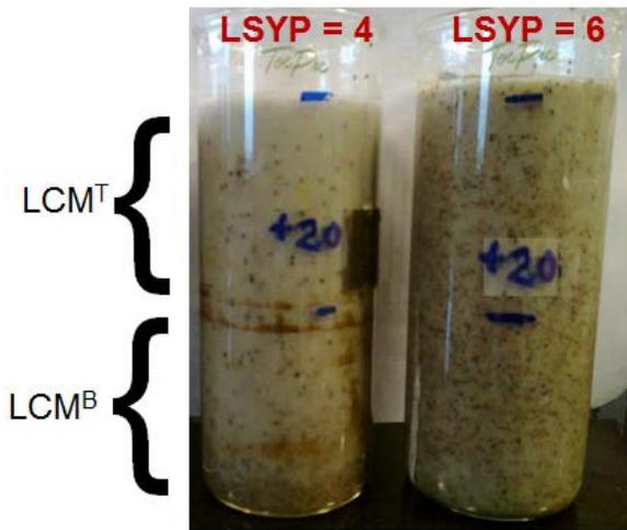
**Figure 2:** Suspension of 850-1000  $\mu\text{m}$  LCM particles (ground walnut particles) in two drilling fluids (fluid *B* and fluid *C*) with variation in LSYP (mud weight= 9.0 ppg).
