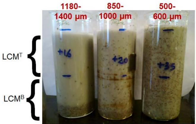
**Figure 1: Suspension of different sizes of LCM particles (ground walnut shells) in water-based Fluid B (9.0 ppg, LSYP = 4).**
