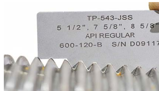
Figure 3: Magnified view of stab flank worn due to fretting, caused by insufficient thread interference.
