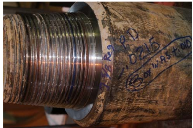
Figure 16: 7 5/8 API Regular displayed evidence of thread fretting. After inspection, it was determined the pin pitch diameter was -.021 ".
