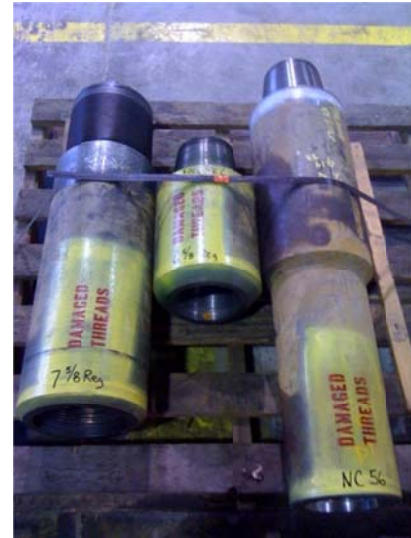
Figure 15: Damaged threads declared by Lewis Inspection Group.
