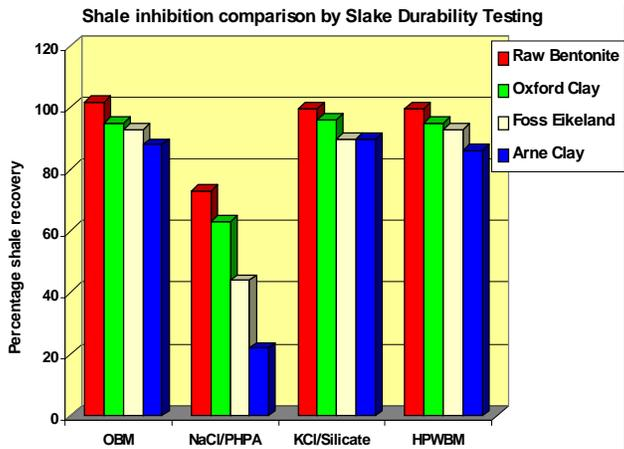
Fig 11 – Results from Slake Durability Test on new HPWBM.
