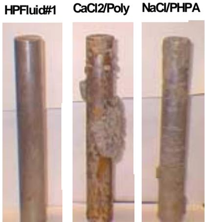
Fig. 9b – Accretion Test pictures from HPWBM development.
