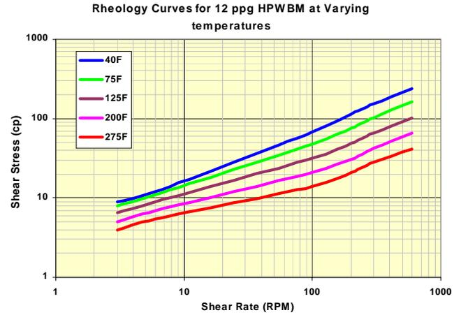
Fig 16 – Rheology curves of new HPWBM over cold-warm temperature range.
