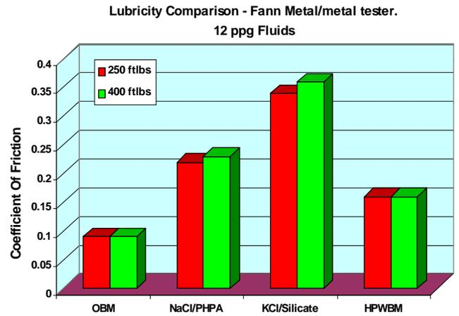
Fig 14 – Lubricity Test results (metal/metal) on new HPWBM.
