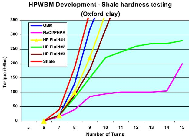
Fig. 8 – Bulk Hardness Test results from HPWBM Development.
