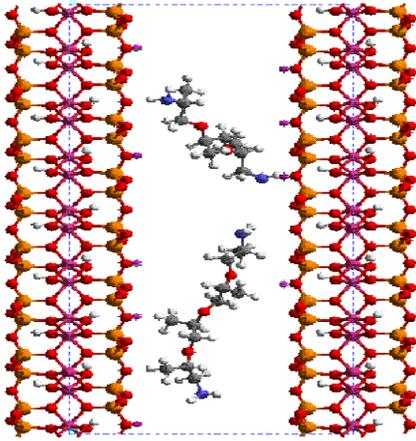
Fig 19 – Molecular modeling results showing binding of hydration suppressant to shale interface.
