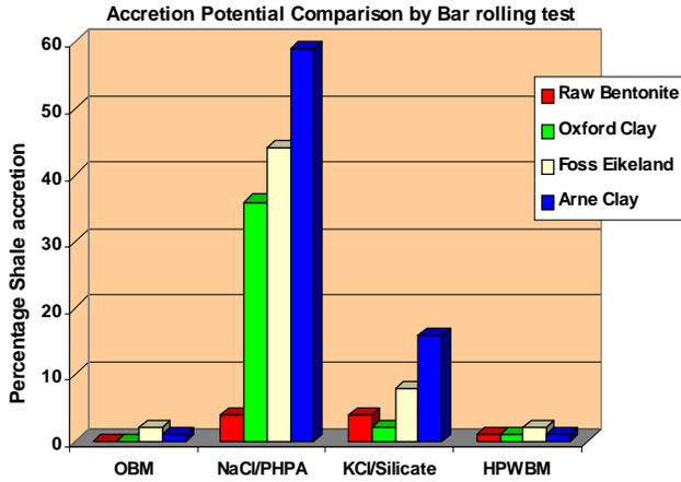
Fig 13 – Results from Rolling Bar Accretion Test on new HPWBM.
