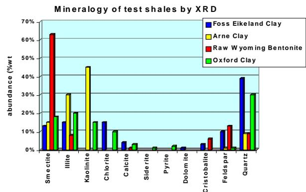
Fig. 1 – Mineralogy by semi-quantitative XRD of the four shale substrates used in laboratory development
