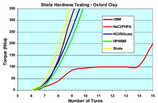
Fig 12 – Results from Shale Hardness Test on new HPWBM.
