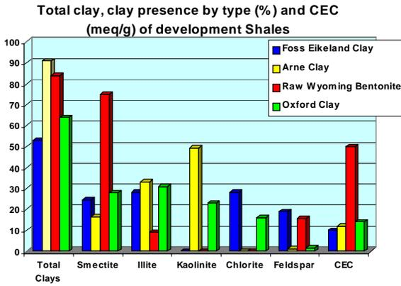
Fig. 2 –Clay content, clay type and reactivity of the four shale substrates used in laboratory development.
