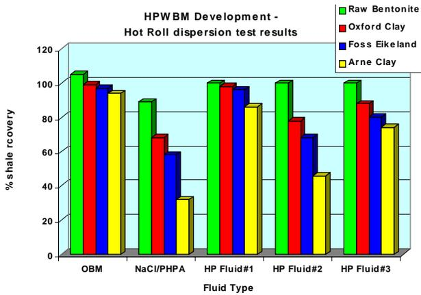
Fig. 4 –Hot Roll Dispersion Test results from HPWBM Development.
