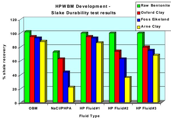
Fig. 6 – Slake Durability Test results from HPWBM development
