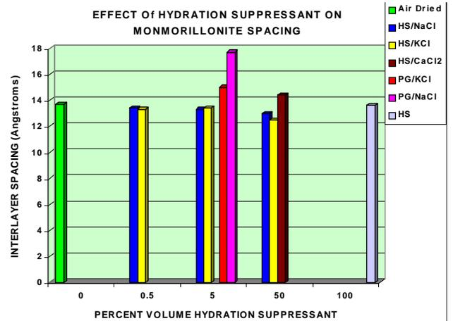
Fig 18 – X-ray diffraction results of clay/salt mixes with hydration suppressant showing interlayer spacing.
