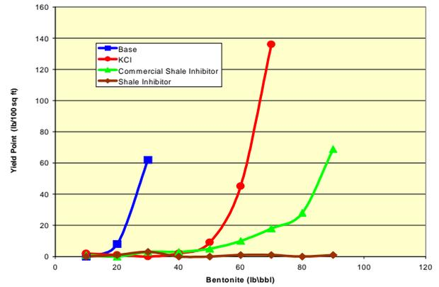
Fig. 3 –Bentonite Inhibition Test comparing the yield point of three shale inhibitors and the base fluid.
