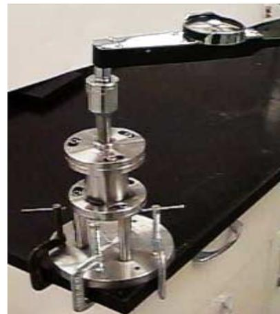
Fig. 7 – Bulk Hardness Tester.
