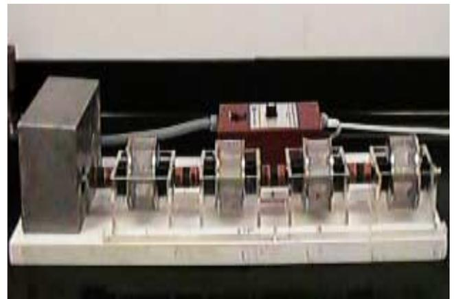
Fig.5 – The Slake Durability apparatus
