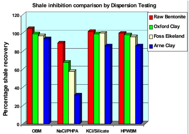
Fig 10 – Results from Hot Roll Dispersion Test on new HPWBM
