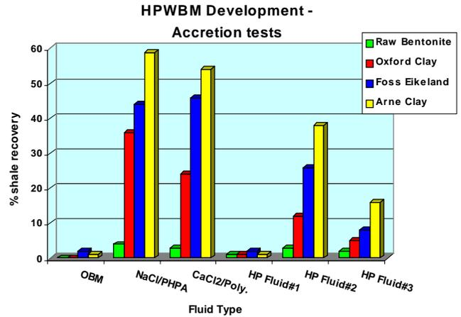
Fig. 9a – Accretion Test results from HPWBM Development.
