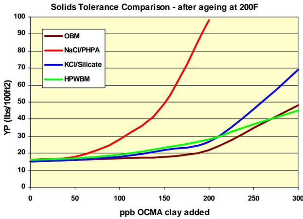
Fig 15 – Results from Solids Tolerance Test on new HPWBM.
