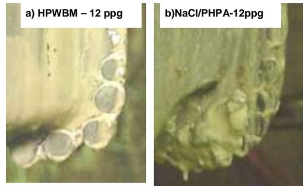
Fig 20c – Full-scale accretion and ROP test results - Photos of bits after a) HPWBM and b) NaCl/PHPA, showing clean cutters in a) and balled cutters in b).
