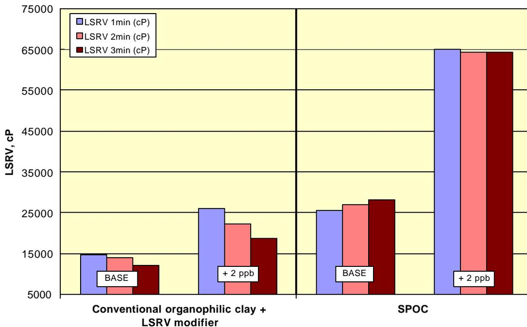
Fig. 2 – Effect of organophilic clays on Brookfield LSRV in laboratory fluids.
