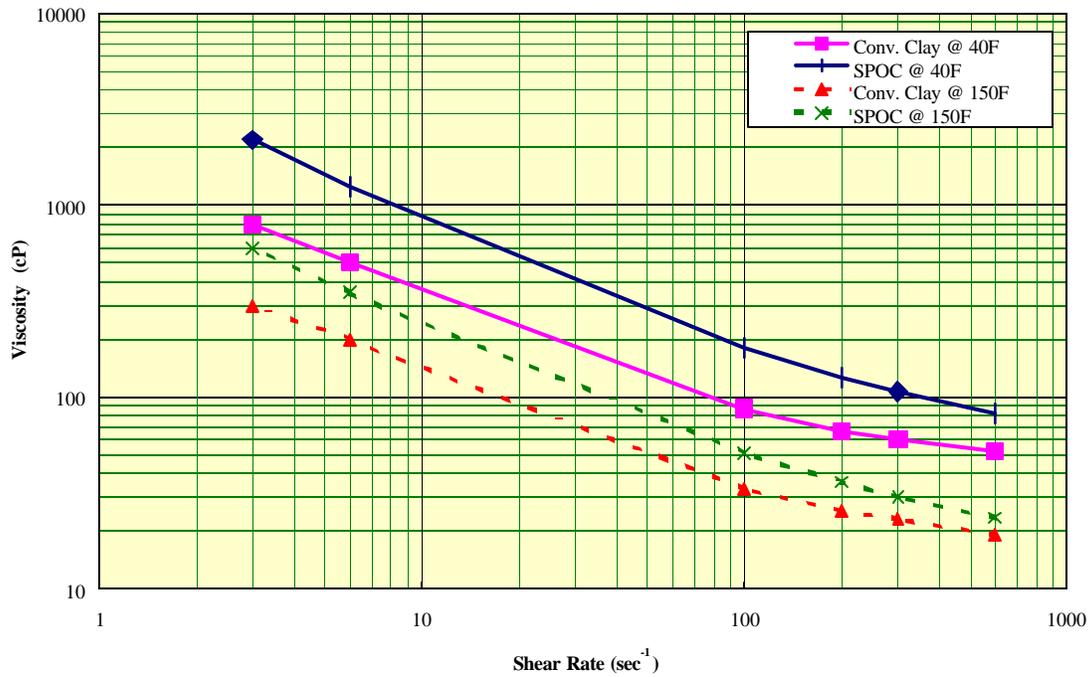
Fig. 3 – Effect of 4-lb/bbl organophilic clays on rheology of SBM at different temperatures.
