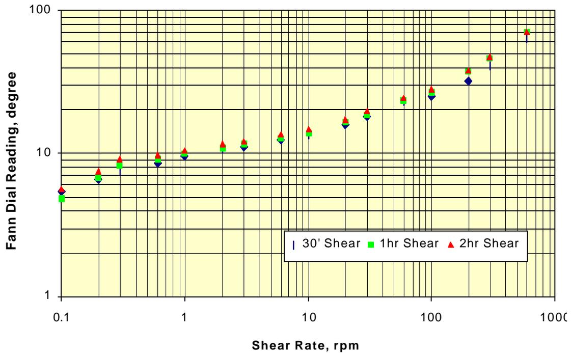
Fig. 6 – Effect of shear on rheology of 14.3-lb/gal SBM treated with 2-lbm/bbl organoclay.
