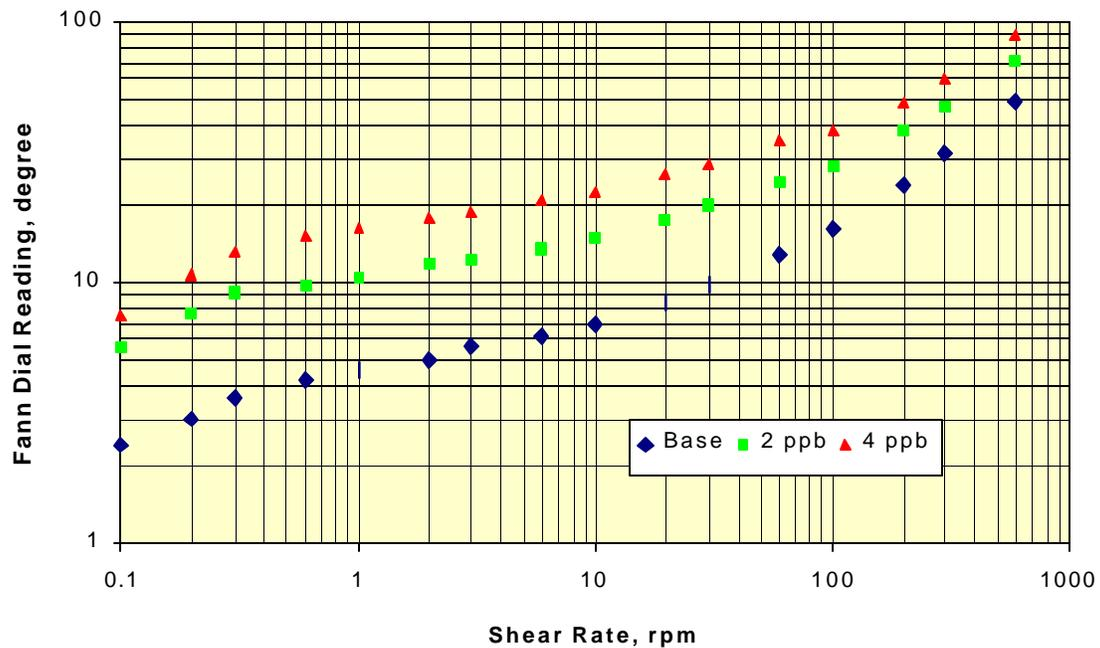
Fig. 8 – Effect of organophilic clay content on rheology of 14.3-lb/gal SBM sheared for 2 hours.
