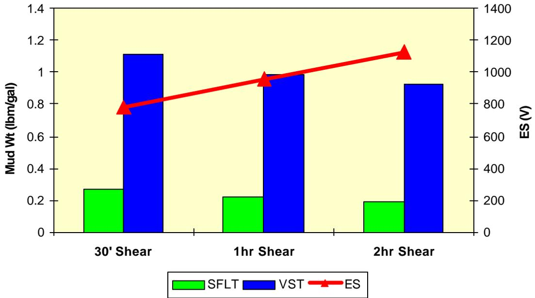
Fig. 5 – Effect of shear on SFLT, VST and ES results.
