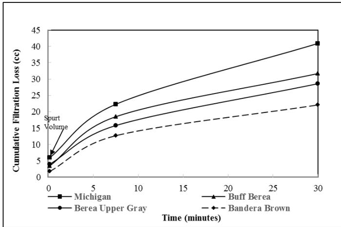
Figure 4. Cumulative filtrate loss using base case water based mud
