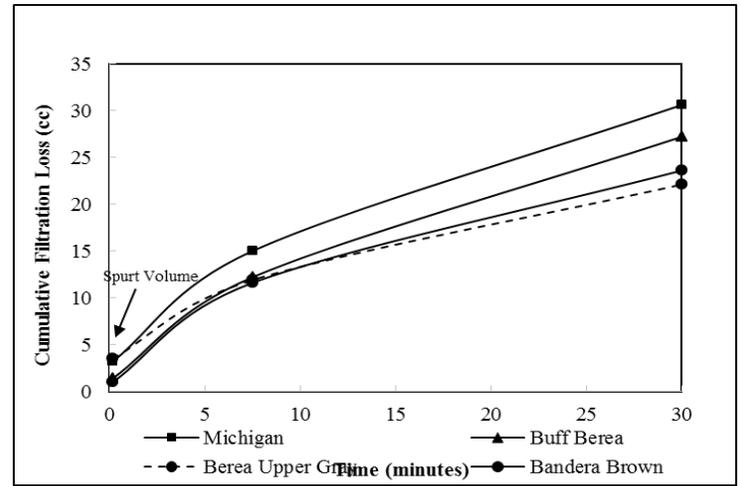
Figure 5. Cumulative filtrate loss using wellbores strengthening water based mud
