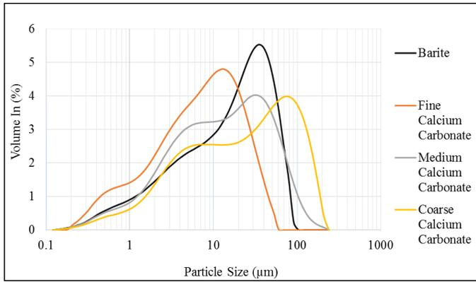
Figure 3. Particle Size Distribution of sized Calcium Carbonate
