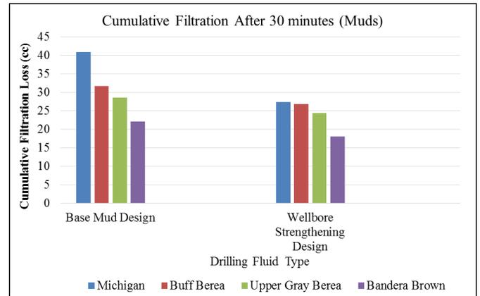
Figure 6. Comparison of cumulative filtrate loss from base design (left) and wellbore strengthening design (right)
