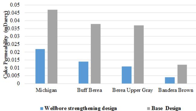
Figure 8. Comparison of mud cake permeability calculated for base design and wellbore strengthening design
