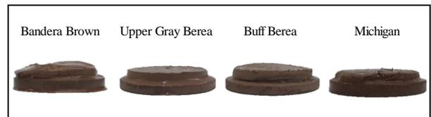
Figure 7. Mud cakes using optimum base design drilling fluid
