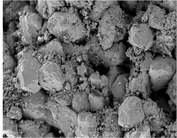
Figure 9. SEM analysis of Michigan core after filtration tests using base case drilling fluids
