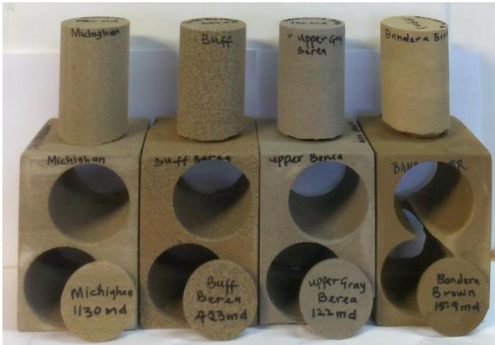
Figure 1: Sandstone slabs used in experiments to prepare rock disks to conduct PPT experiments
