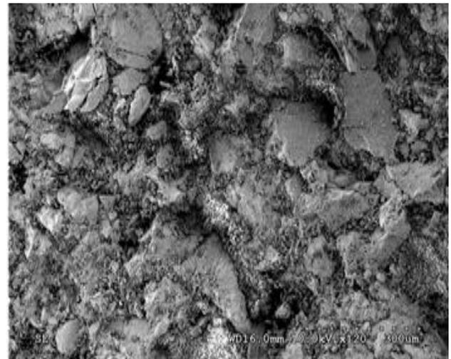
Figure 10. SEM analysis of Michigan core after filtration tests using wellbore strengthening fluid's design
