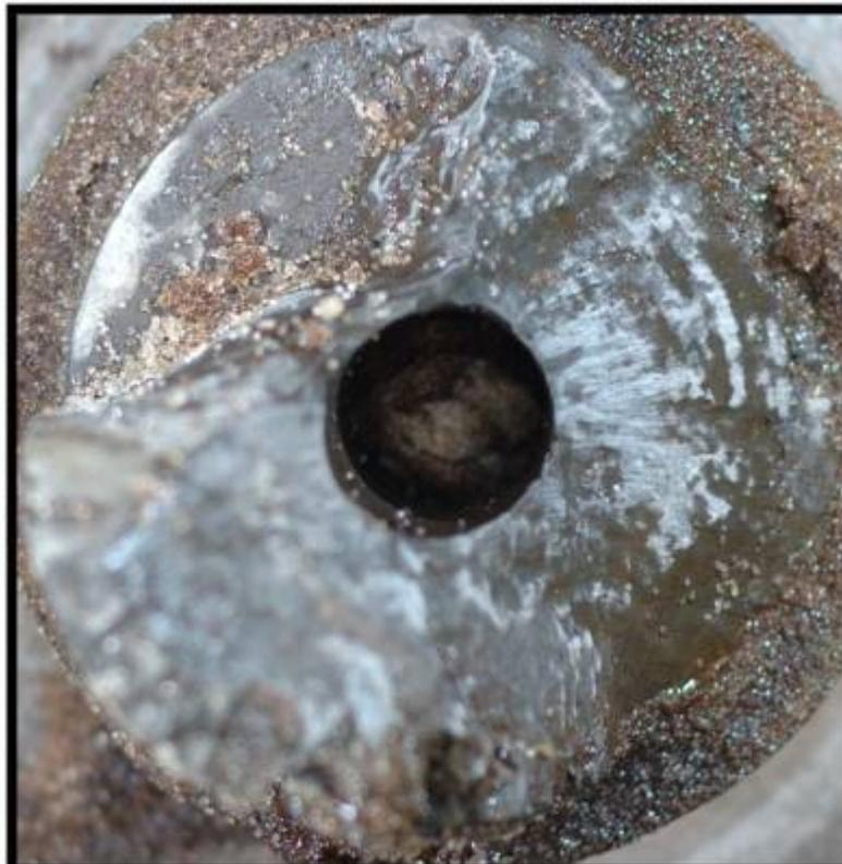
**Photo 2 - Shallow Pleistocene shale drilled with 0.5 Aw oil mud**
