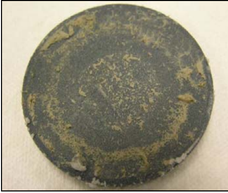
Figure 9 OBM filter cake after treatment with SPME + formic acid
