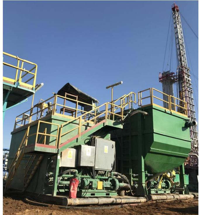
Fig. 01 – High-Volume Dewatering System.
