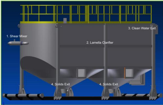
Fig. 5 - High-Volume Dewatering System Separation Module Process Flow
