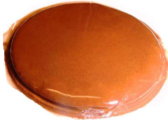
Figure 5. Filter cake (<1mm) of Mn 3 O 4 in KFo fluid that was heat aged for 30h at 400°F and filtrated statically at 300°F and 500psi.
