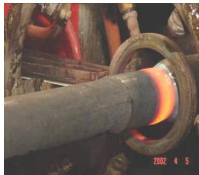
Figure 5. Example of Drill Pipe friction weld under heat treatment.
