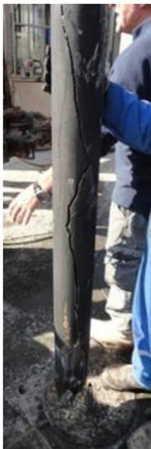
Figure 4. Example of cracked Drill Pipe after H<sub>2</sub>S exposure in North Iraq.
