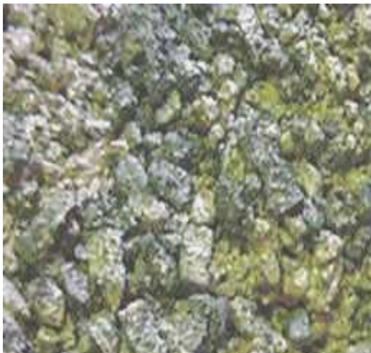
Picture 1 – Picture of shale cuttings drilled with new polymer fluid and K 2 CO 3 , showing bit marks on overall large, well inhibited cuttings.
