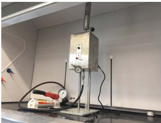
Figure 3- HPHT PPA with LCM Receiver
