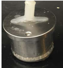
Figure 6- Effectively Sealed Tapered Disc by the Smart LCMs.
