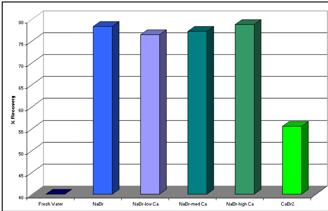
Figure 2: Effect of Brine Type on Shale Dispersion
