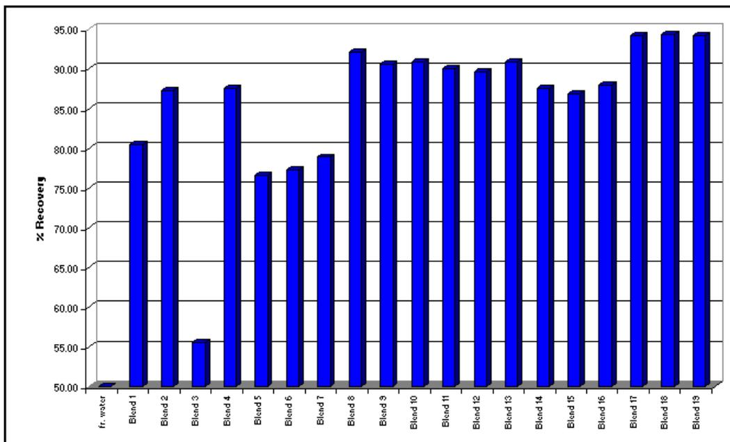
Figure 1: Shale Dispersion Testing—All Fluids
