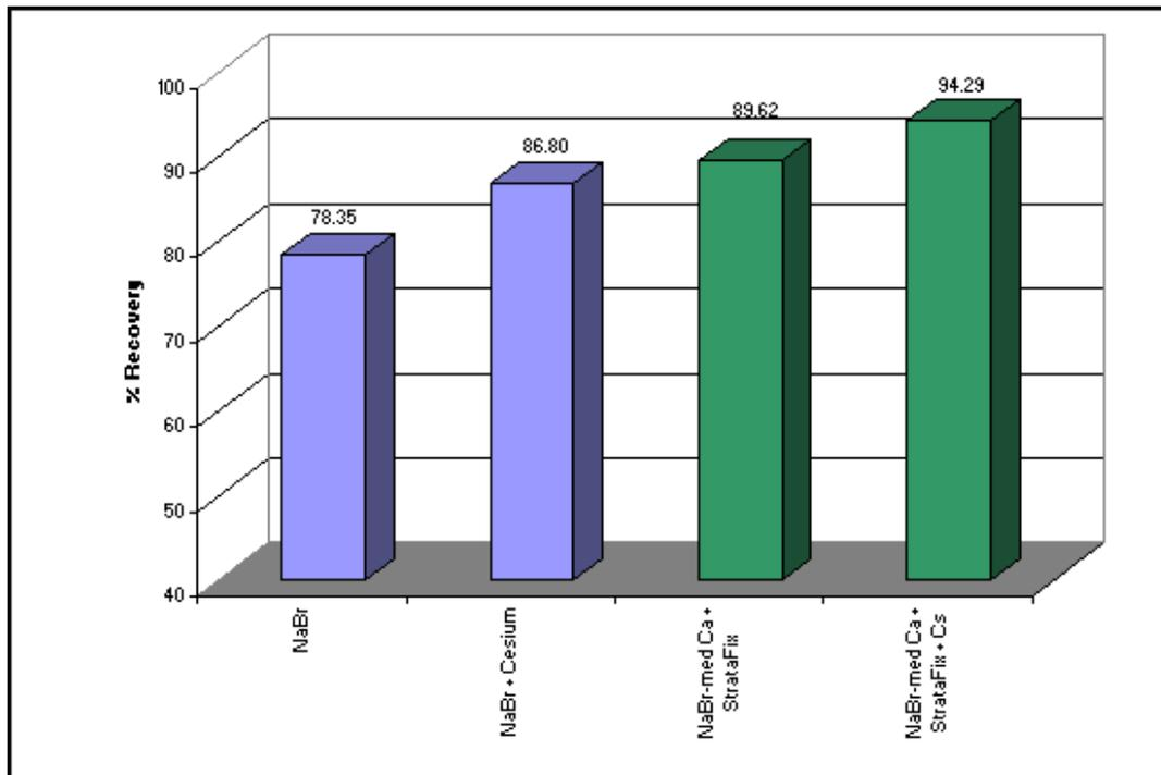
Figure 4: Effect of Cesium Formate on Shale Dispersion
