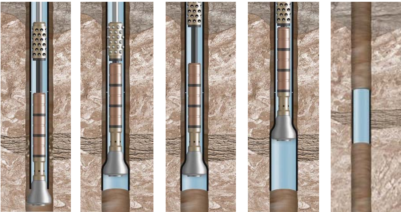
Figure 2 – Running sequence for the single-diameter openhole clad system.
