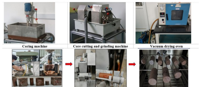
Figure 3 - Core processing flow chart and physical images
