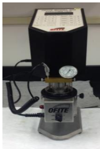
Figure 2: Rotational viscometer used to obtain rheological parameters of drilling fluids.
