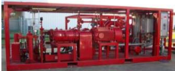
**Rig Pump Diverter (RPD)** – evolved from BPP lessons learned and diverts flow from existing rig pumps away from stand pipe and down the drillstring to across the annulus into the MPD flowline and across the automated choke(s), providing continuous non-interrupted flow during multiple operations. This automated approach is key to precise BHP during these operations.
