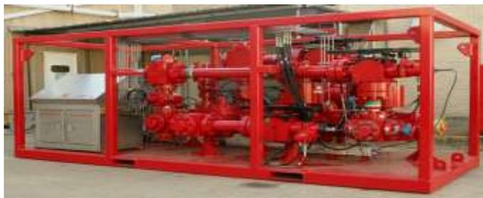
**Backpressure Pump (BPP)** – first-generation MPD required the use of BPP to supply continuous flow across flow across the chokes for BHP control.
