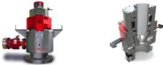
**Automated MPD Choke** – is the pressure regulator in the closed-loop control system throughout all operations, including drilling, tripping, casing running, and cementing operations. The system also incorporates a mass flow (Coriolis) meter for continuous measurement of rate and density of the return fluid, which aids in precise BHP control and event detection.
