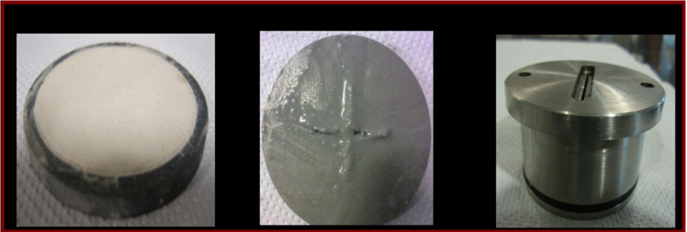
Figure 2: Different filtration medium used for loss circulation treatment design for permeable section and fractures.
