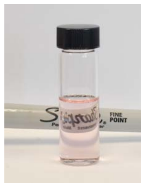
Fig. 3–15 volume-% diesel solubilized in an 80:20 mixture of brine/surfactant mixture.
