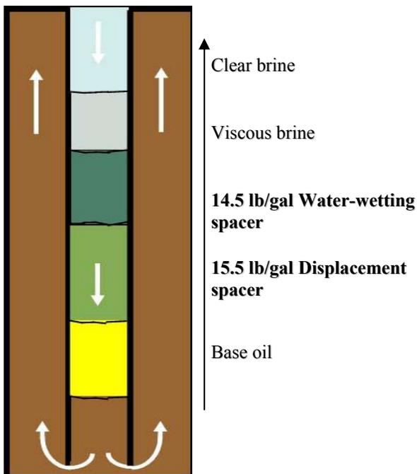
Figure 5. Sequence of fluids displacements
