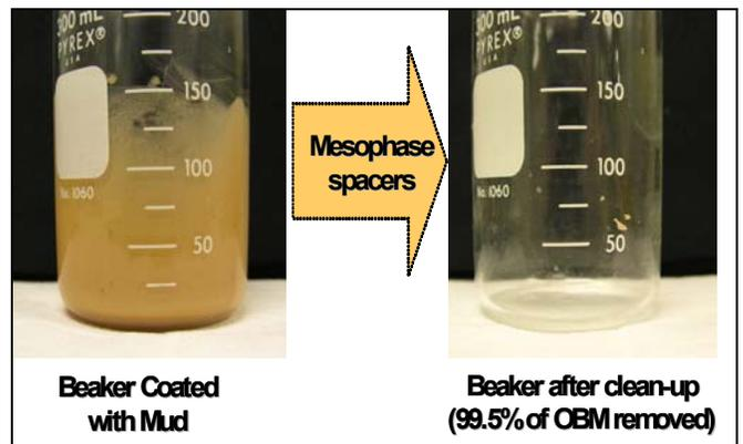
**Figure 3. Cleaning test in a beaker**
