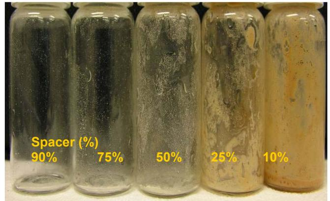
**Figure 2. Final step of vial test: rinse with water**
