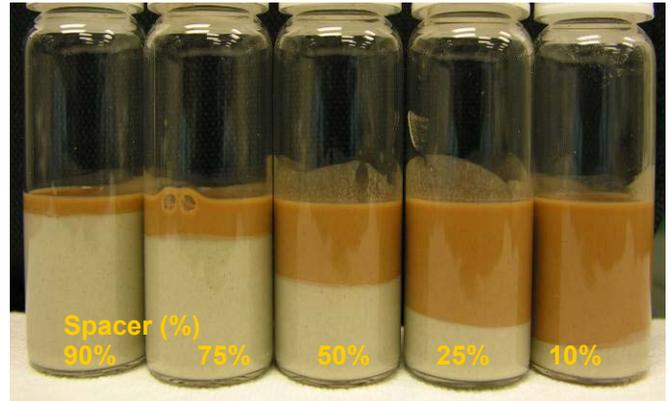
**Figure 1. Initial step of vial test: SBM poured on top of spacer**
