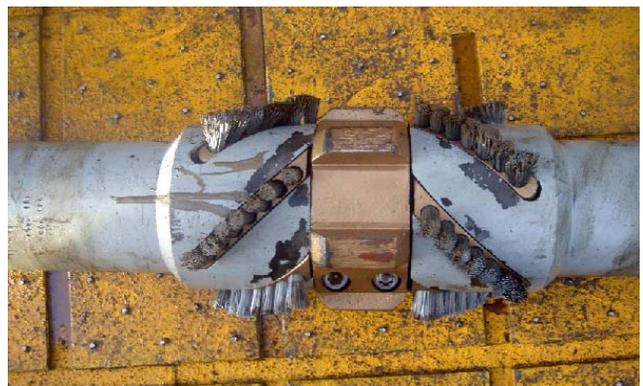
Figure 8. Photograph of casing brush after displacement
