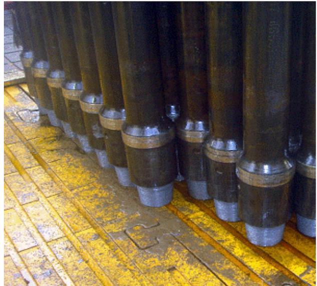
Figure 7. Photograph of clean drill pipe and tool joints after displacement
