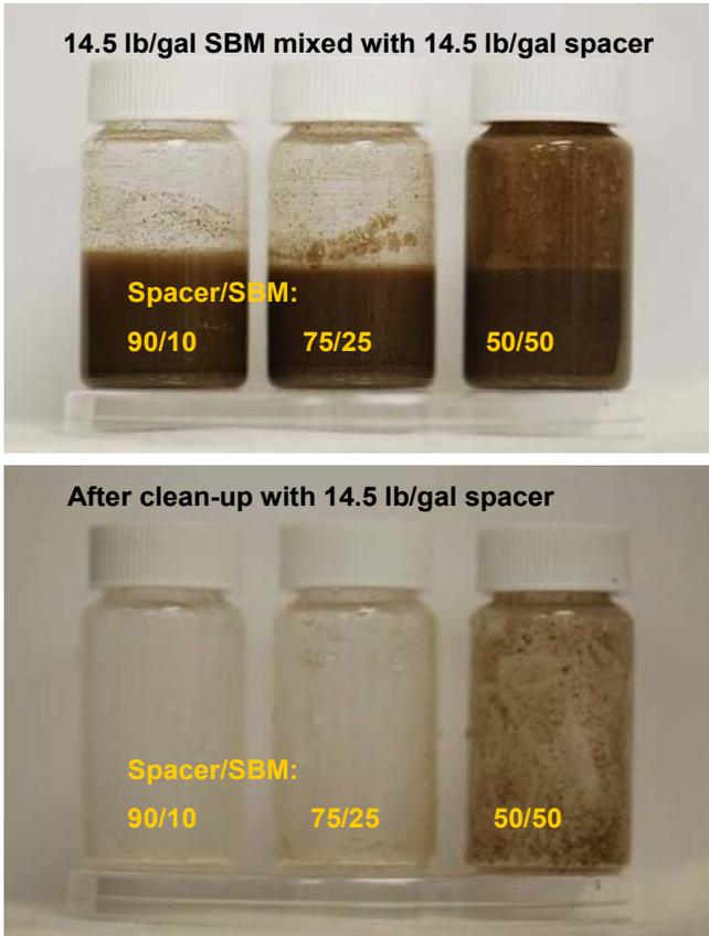
Figure 4. Clean-up test of SBM from OCS-G 25103 well with water-wetting spacer
