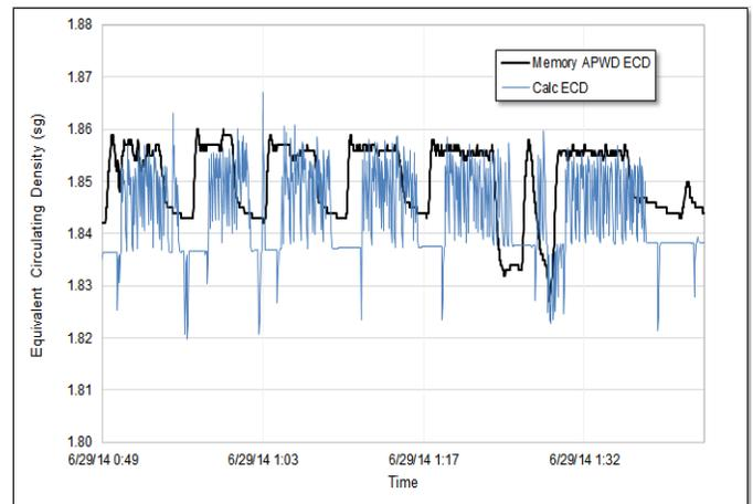
**Fig. 6.** Comparison of APWD ECD memory data and RTHM software while tripping in the hole after recovering the APWD memory data.
