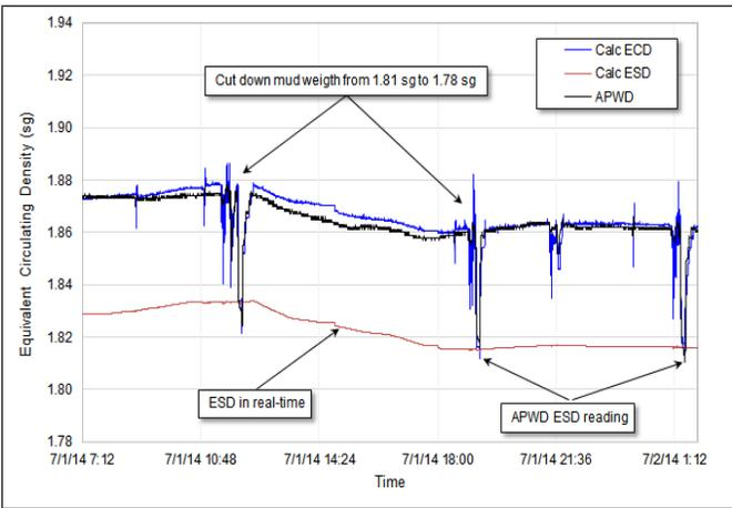
**Fig. 3.** The RTHM software performs ESD calculations in real time, and the results are compared every connection against the APWD.
