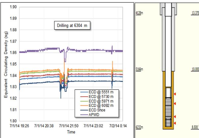
**Fig. 4.** Different points of interest are monitored in real time in addition to the ECD at the APWD's position. Five points of interest are monitored (i.e., a week sand below the casing shoe).
