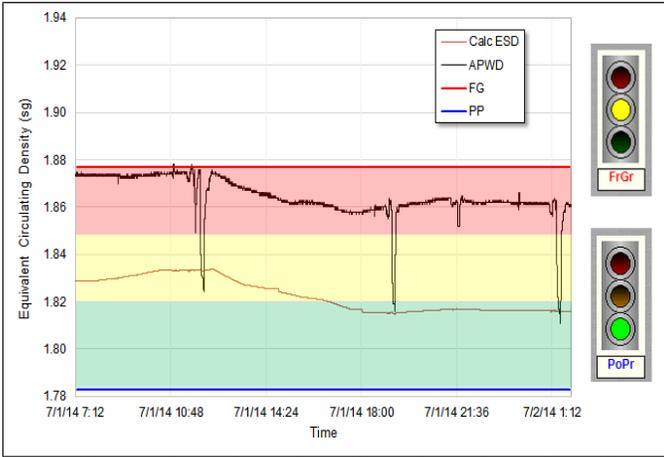
**Fig. 8.** The RTHM software display uses a traffic light format to indicate how close or far are we to the FG/PP.
