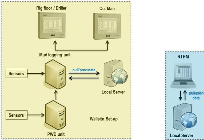
**Fig. 2.** Basic RTHM software configuration for remote communications. All calculations are performed onshore.
