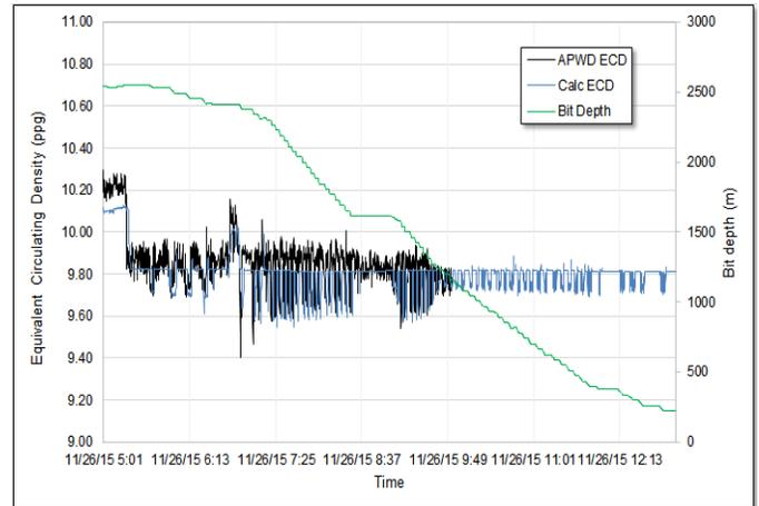
**Fig. 5.** Comparison of APWD ECD memory data and RTHM software while pulling out of the hole after the APWD memory data is recovered.
