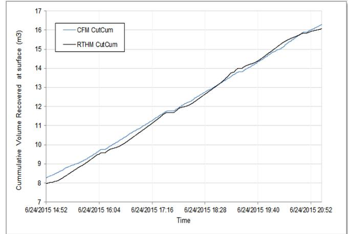
**Fig. 11.** The RTHM software calculates the cumulative volume recovered at surface, this can be compared vs the actual volume in order to determine if cuttings are remaining in the well or not.
