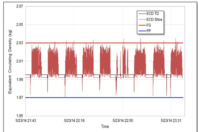
**Fig. 7.** A surge casing run monitored with the RTHM software managing the calculated ECD between 1.97/2.03 sg PP/FG. As measurement to prevent mud losses.
