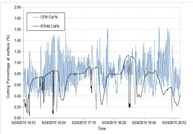
**Fig. 10.** Using the CFM technology, the cuttings concentration at surface can be compared against the calculated cuttings concentration.
