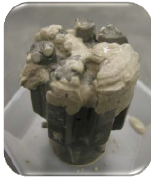
Fig. 5 – Balled bit after completing ADS test.
