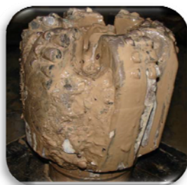
Fig. 1- PDC bit balling in carbonates
