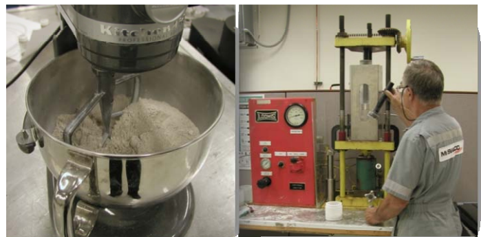
Fig. 3 – Blending and compacting formation samples.
