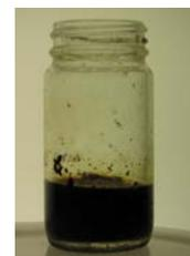
**Fig. 2 Scavenger A aged with 12.5 NaBr brine for 16 hours at 300°F**
