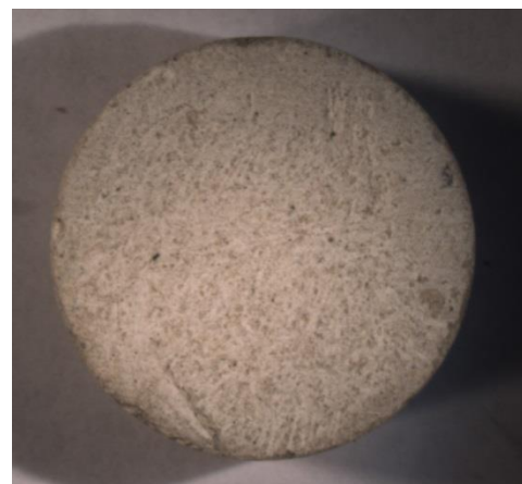
Figure 2, class F fly ash: AAAS:Fly Ash: Zn- polyethylene glycol slurry, ~ 17% expansion
