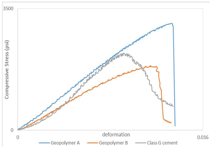
Fig. 6: Compressive stress vs deformation for Geopolymer A and B and Class G cement cured at 200°F
