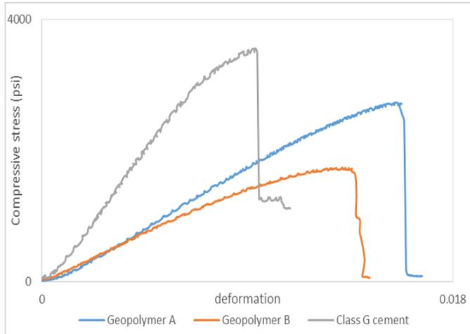
Fig. 5: Compressive stress vs deformation for Geopolymer A and B and Class G cement cured at 150°F
