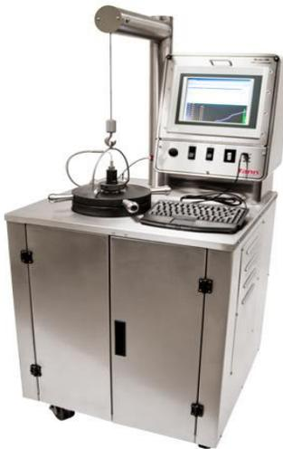
Figure 8: HPHT consistometer set up used for measuring geopolymer thickening time
