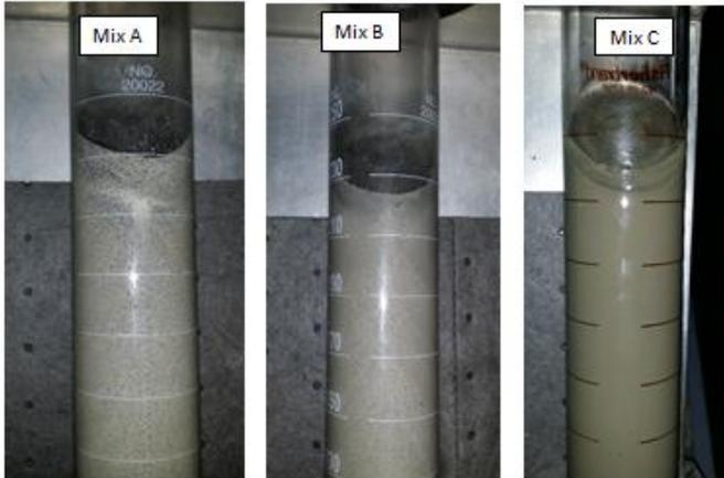
Figure 3. Detailed view of the free fluid test
