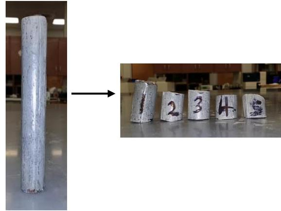
Figure 4. Fly ash geopolymer cured at 150°F and 3000psi divided into 5 unequal portions
