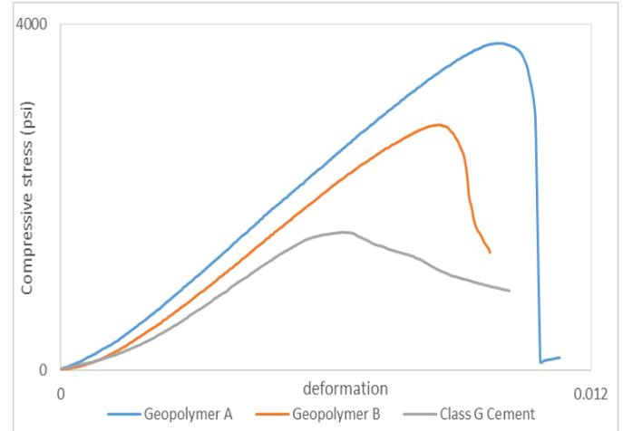
Fig. 7: Compressive stress vs deformation for Geopolymer A and B and Class G cement cured at 250°F
