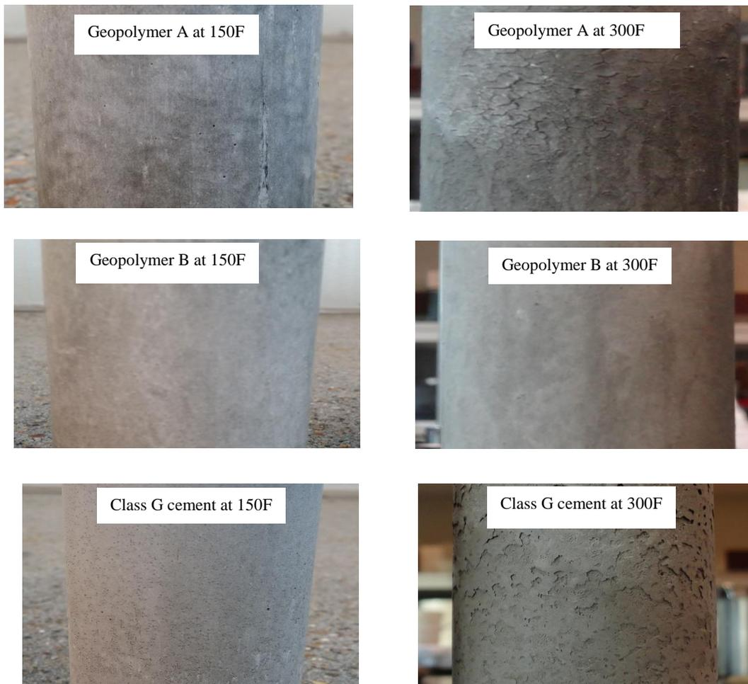
*Fig 2: Surface of Geopolymer A and B and Class G cement at 150°F and 300°F*
