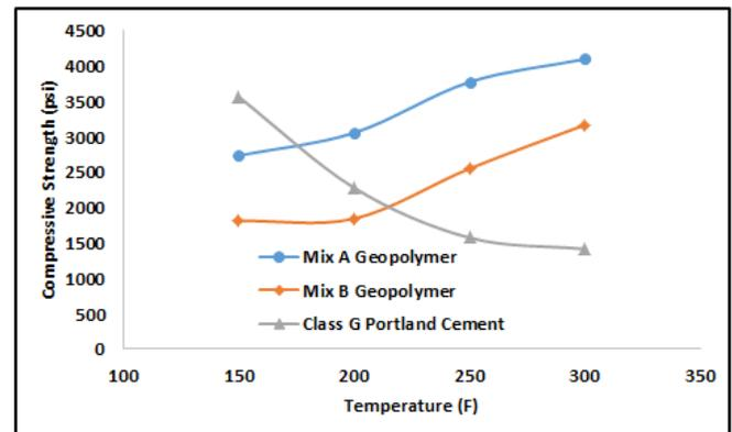
Fig. 1: Compressive strength development at various curing temperature
