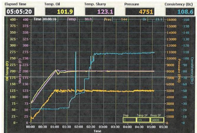
Figure 10: Thickening time results for the optimized sample using suitable mix of plasticizer (5 hrs)
