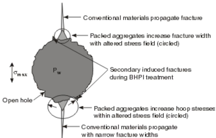
Fig. 6—Secondary induced fractures *during* BHPI treatment.
