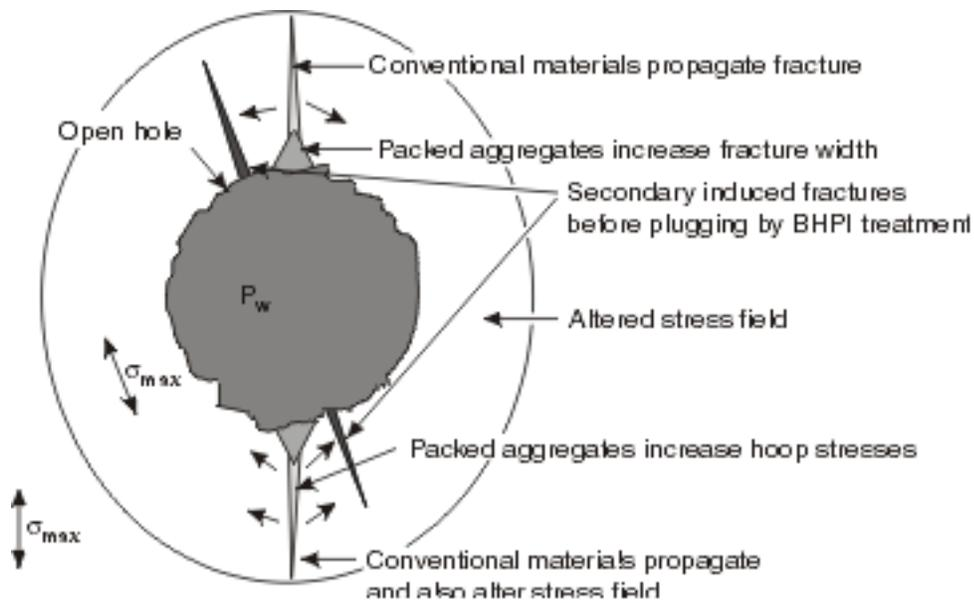
Fig. 5—Secondary induced fractures *before* plugging by BHPI treatment.
