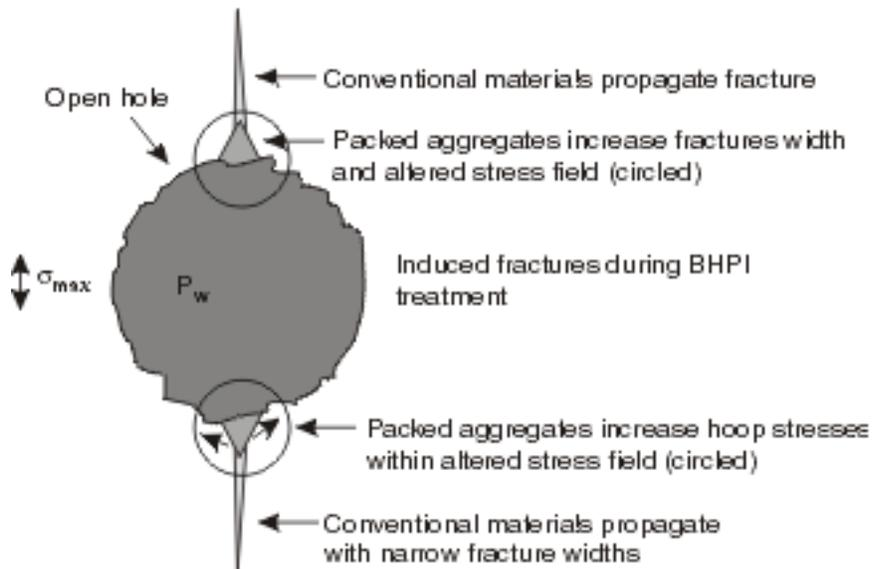
Fig. 4—Induced fractures during BHPI treatment.
