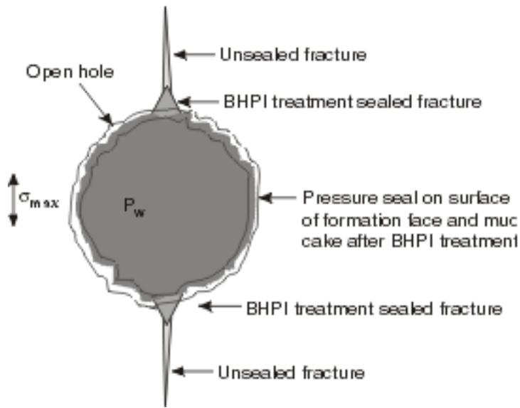
Fig. 3—Pressure seal on formation face and mud cake after BHPI treatment.
