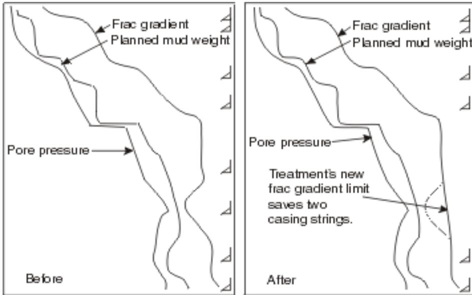
Fig. 1—Balancing pore pressure and frac gradient.
