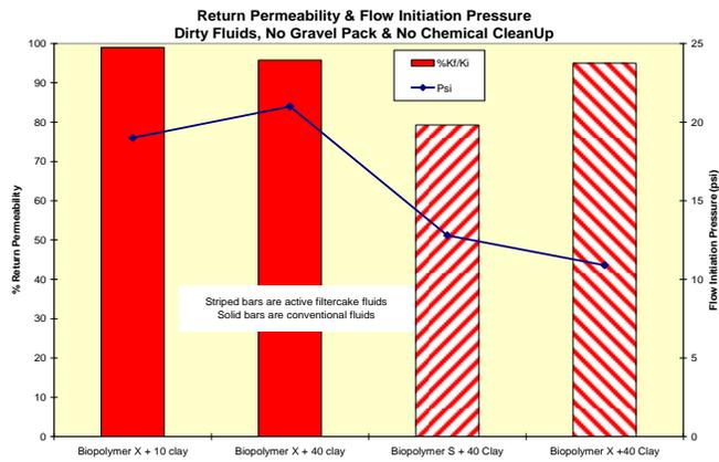
Figure 2 – Virgin Conventional RDF (solid bar) and SFC (striped bar) Systems with 40-lb/bbl OCMA clay.
