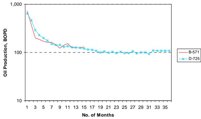
Figure 7 – Comparison in oil production between SFC (B-571) and DIF (D-725) RDF systems.
