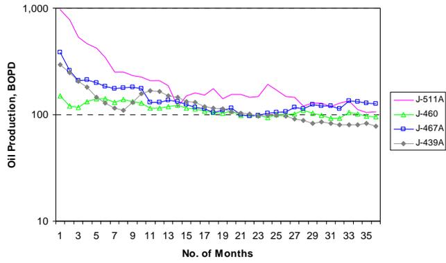
Figure 6 – Comparing SCF RDF (J-511A) crude production vs. three selected conventional RDF systems.
