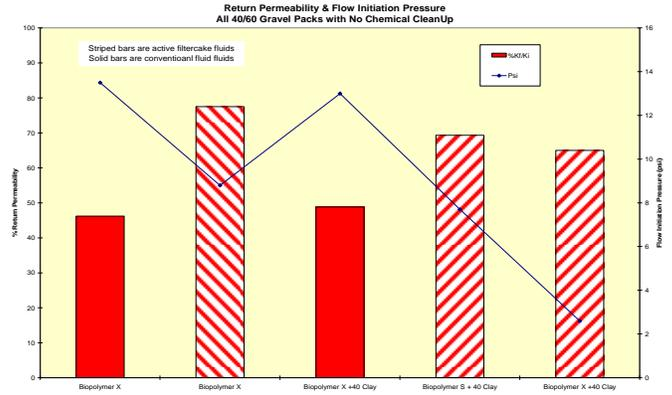
Figure 3 – Virgin Conventional RDF (solid bar) and SFC (striped bar) Systems with 40/60 sand and screen.
