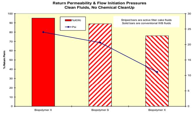
Figure 1 – Virgin Conventional RDF (solid bar) and SFC (striped bar) Systems.
