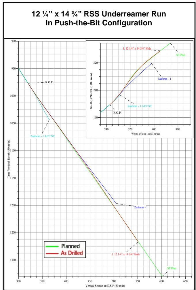
Figure 6: Comparison plot of Planned (green) versus Actual (red) wellpath.
