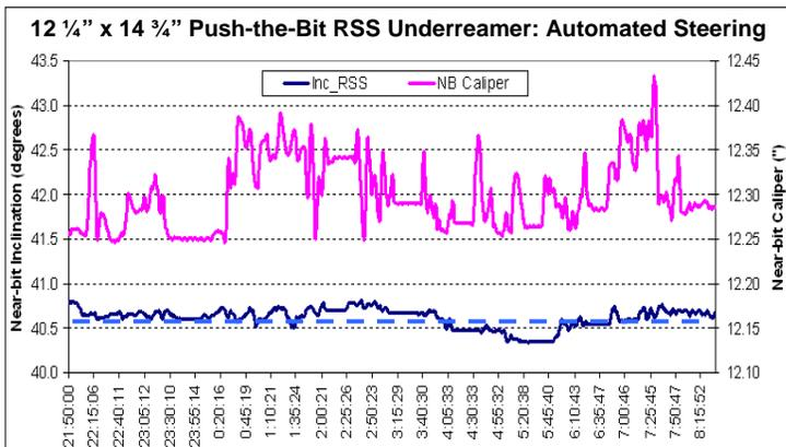
**Figure 8:** Automated Hold Mode was used in the tangent section at 40.6°.
