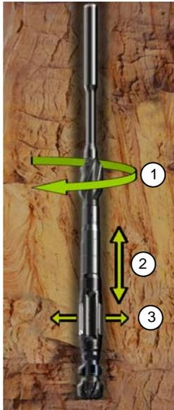
**Figure 2:** Typical Downhole Vibration — 1) torsional, 2) axial, and 3) lateral.
