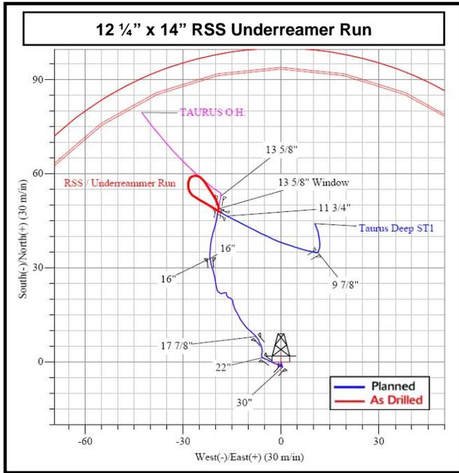
Figure 5: Comparison plot of Planned (blue) versus Actual (red) wellpath
