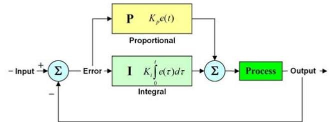
**Figure 1:** An example control algorithm
