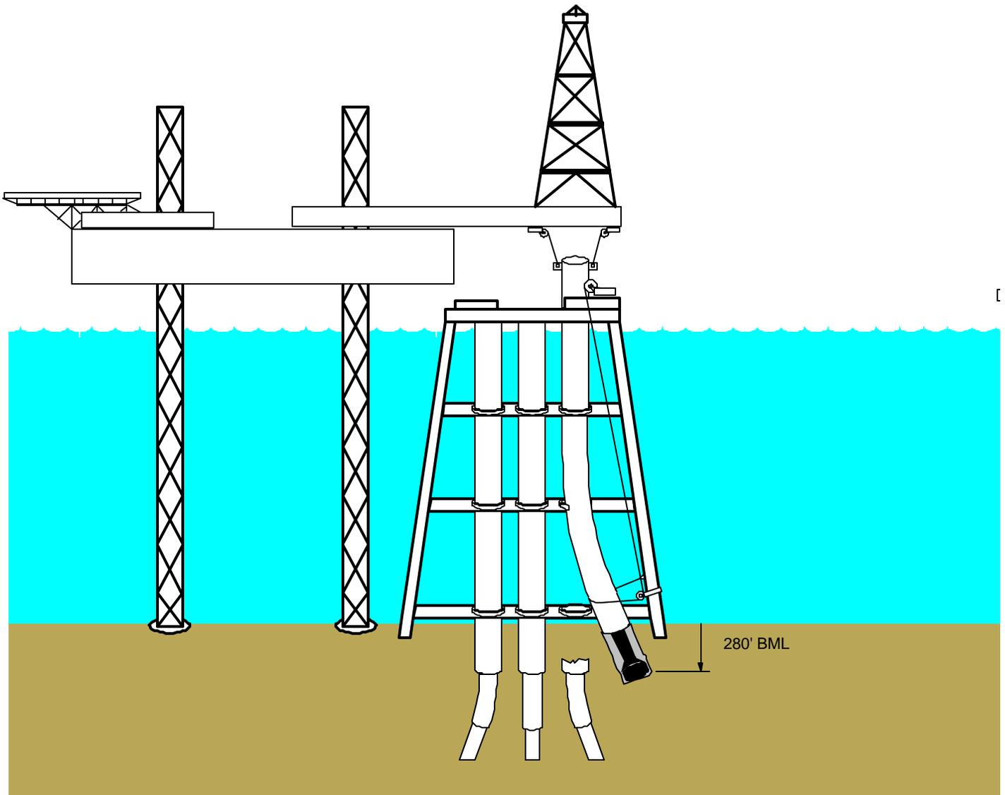
**Drill out below new drive pipe with rotary jetting bha to 280' BML without NU a diverter.**
