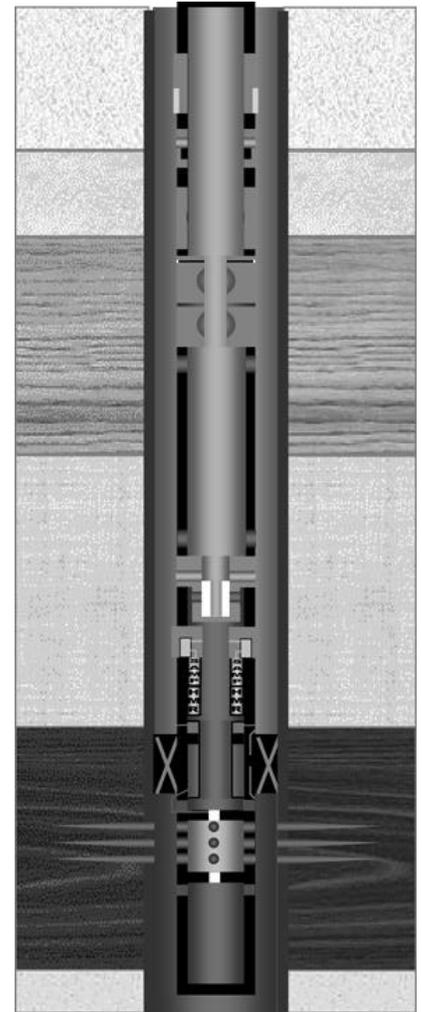
**Fig. 8 — Circulating the well.**
