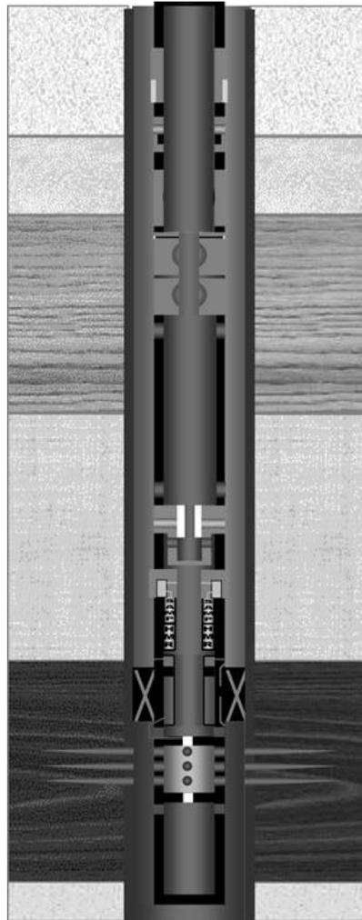
**Fig. 7 — Annulus pressure is reapplied to open the upper surge valve, starting the third surge/flow period. Well is circulated, and a large volume sample is recovered at surface.**
