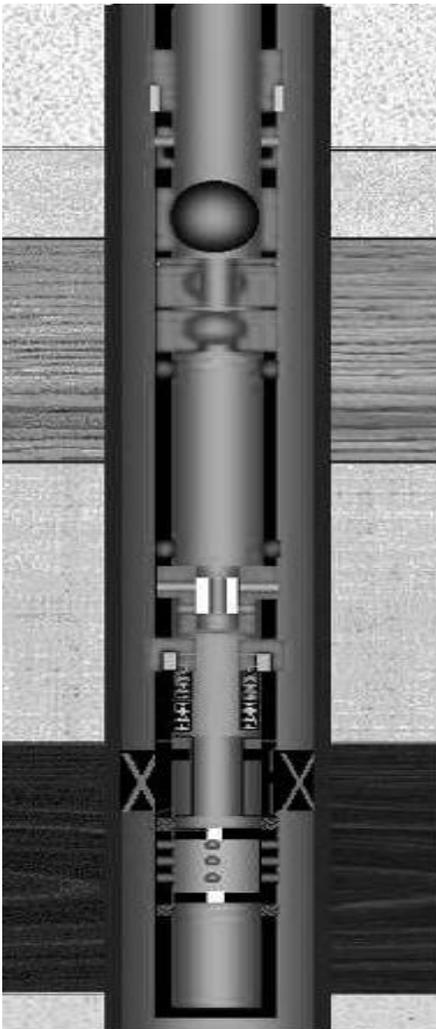
**Fig. 3 — Annulus pressure is applied to activate the firing head and open top and bottom flow vents, allowing junk and mud to go to the lower chamber.**
