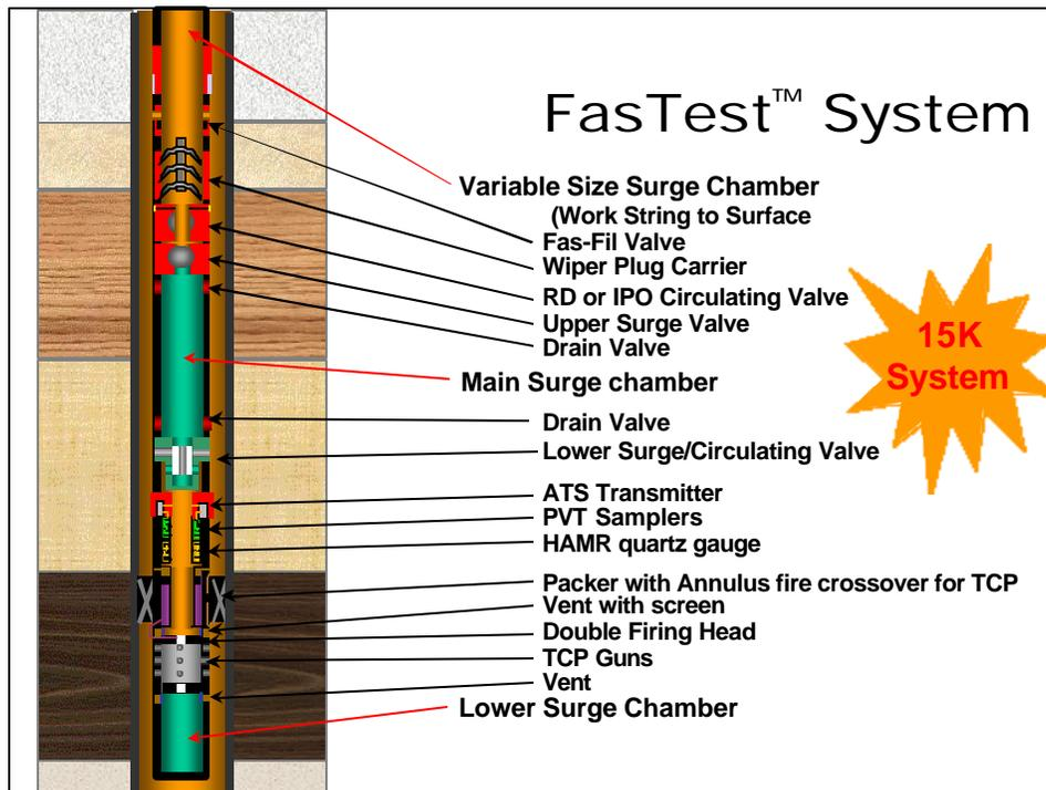
Fig. 2 - Configuration of the system.
