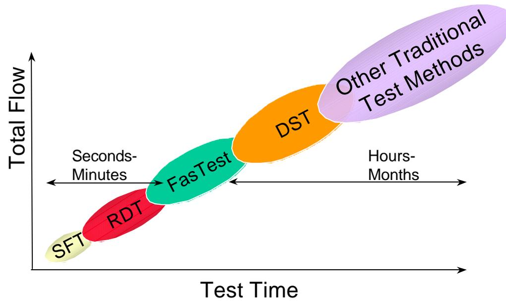
Fig. 9 — Emission free sampling and testing method in relation to other methods.
