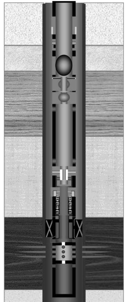
**Fig. 5 — Starting Initial surge and pressure build-up period.**
