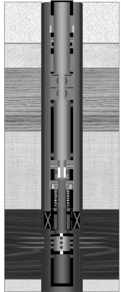
**Fig. 8 — Circulating the well.**
