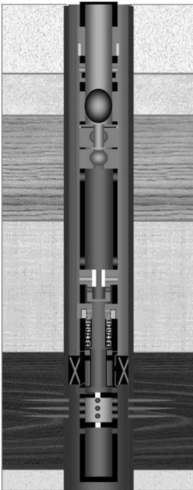
**Fig. 6 — Annulus pressure is reapplied to shift the lower surge/circulating valve to the well test position, starting the second surge and shut in period .**
