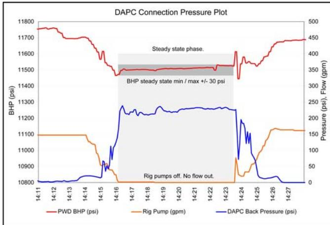
Figure 6 – pressure plot example showing steady state window during a connection.
