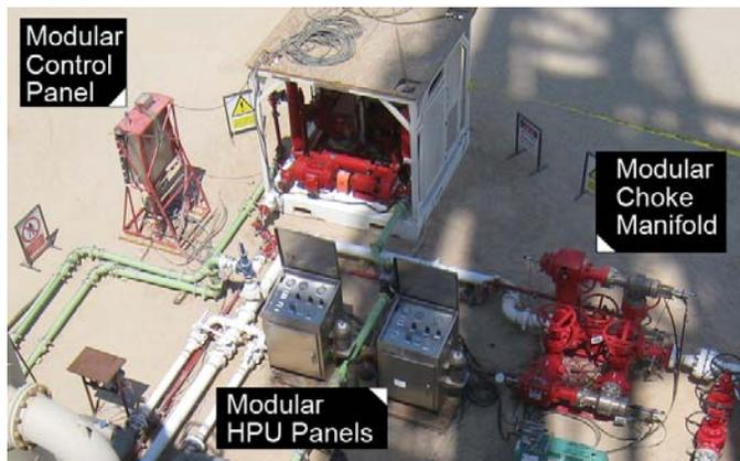
Figure 3 - photo of a modular DAPC choke manifold.
