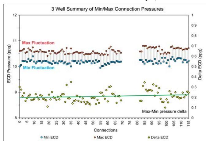
Figure 11 – summary of minimum and maximum pressures managed by the DAPC system during 115 connections, 109 of which (95%) of which were within a  $\pm 0.3$  ppg window relative to a 10.5 ppg setpoint. The green line represents the average trend of min/max pressure delta over the 3 wells.
