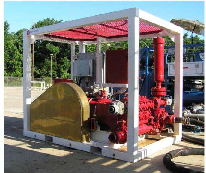
Figure 4 - photo of a DAPC back pressure pump.
