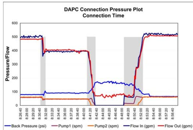
Figure 15 – pressure plot highlighting several dynamic transient periods including a sudden drop in flow and the pump transitions before and after the connection.
