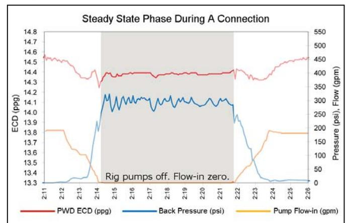
Figure 5 - plot of pressure and flow managed by the DAPC system during a connection showing the phase defined as steady state.
