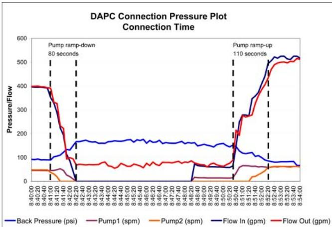
Figure 17 – a detail look at the pump transitions before and after the connection and their duration.
