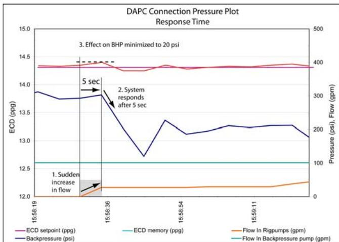
Figure 13 – same pressure plot as in figure 12 with expanded time scale to show the details of the transient event.
