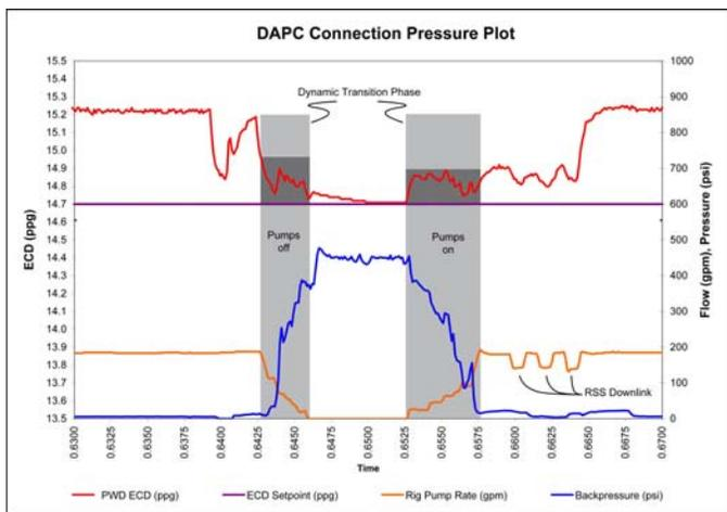
Figure 10 – the same pressure plot as shown in figure 8 highlighting the BHP fluctuations that occur as recorded by the PWD tool during the dynamic transition.
