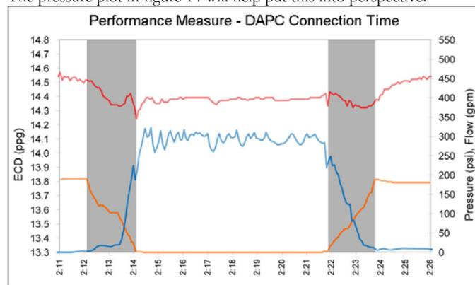
Figure 14 – pressure plot highlighting the MPD connection time which coincides with the transient periods prior to and after a connection.
