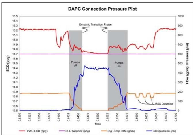
Figure 9 – plot of pressure managed by the DAPC system during a connection showing the dynamic transition phase during which the rig pump is being turned off and on.
