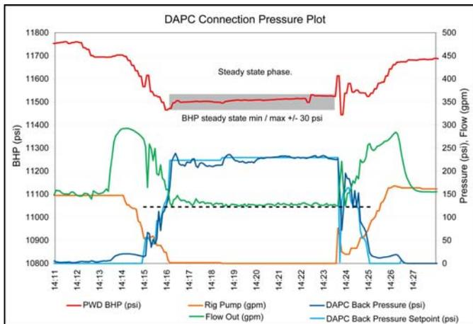
Figure 7 – the same pressure plot example as shown in figure 6 of a steady state during a connection showing a slight amount of flow-back as indicated by the flow-out curve just after the rig pump was turned off.
