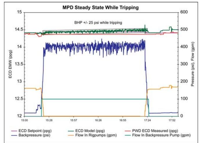
Figure 8 – pressure plot example showing a steady state phase and pressure window while tripping out of a well.
