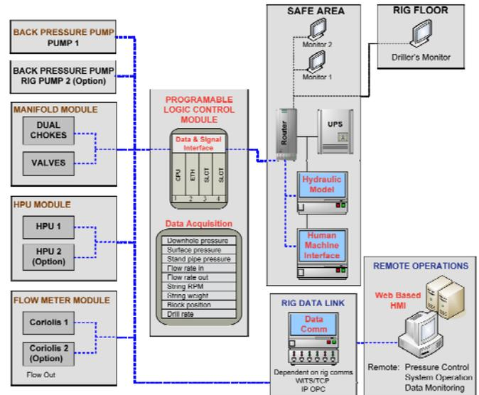
Figure 1 - schematic of DAPC integrated control system.
