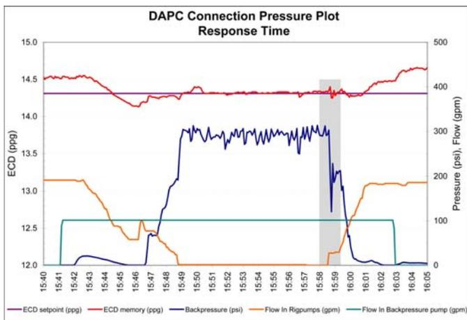
Figure 12 – pressure plot highlighting a transient pressure event caused by sudden increase in the flow rate immediately after the connection.
