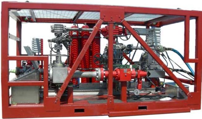
Figure 2 - photo of a self-contained DAPC choke manifold.
