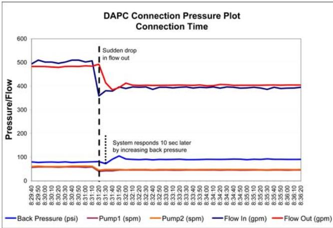
Figure 16 – a detail look at the sudden drop in flow just prior to the connection.
