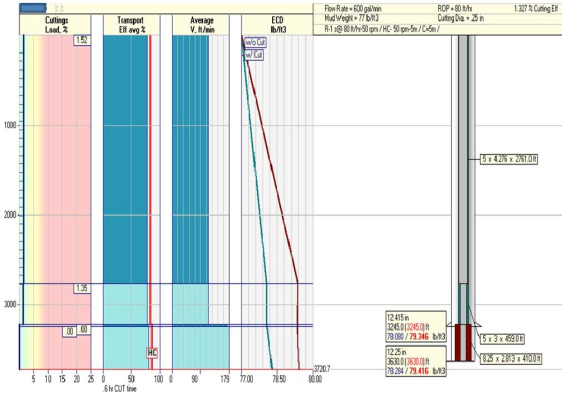
Fig. 1—Graph of the drilling simulation to determine optimum hole cleaning parameters with the advanced hydraulics software.
