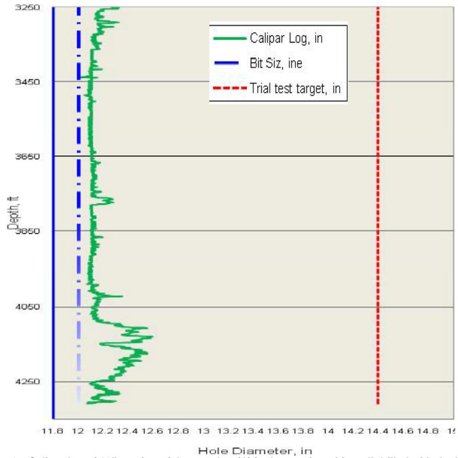
Fig. 3—Caliper log of 12” section of the member (A) in the stratigraphic well drilled with the HPWBM.
