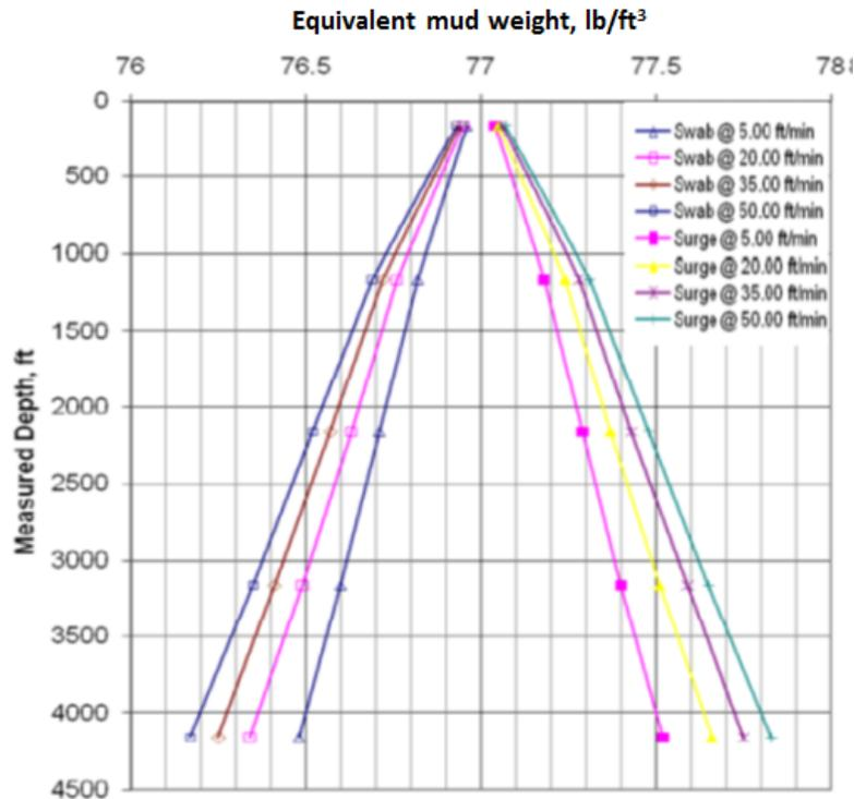
Fig. 2—Graph from advanced hydraulics software showing surge and swab pressures used to determine optimum tripping speeds in and out of the hole.
