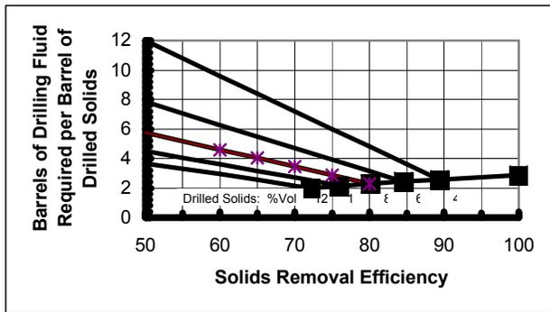
Effect of Targeted Drilled Solids Concentration on Discard Volume
