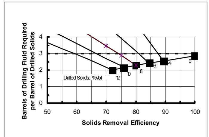
Comparison of Drilling Fluid Volume required with Rule of Thumb of "3"
