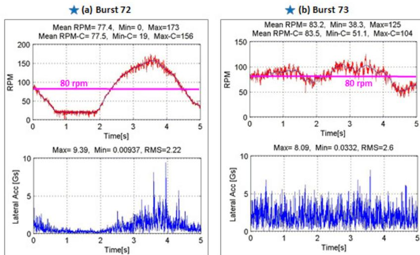
Figure 10: Well A – Burst Plots in Stick-Slip (a) and Whirl (b)
