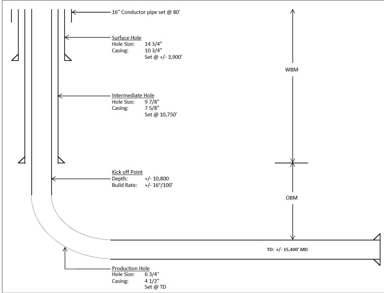
**Figure 3:** Casing Design for Project Wells A and B
