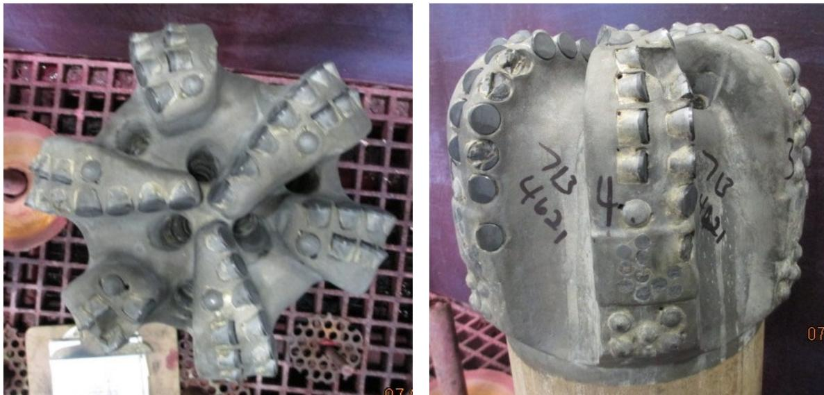
Figure 16: Well A – Second 9.875-in PDC Bit with Six Blades and 16mm Cutters
