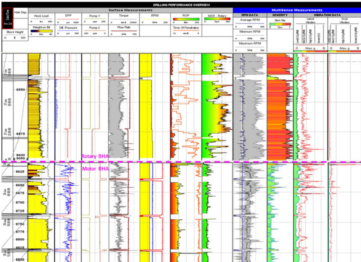
Figure 14: Well A – BHA Change from Rotary to Motor
