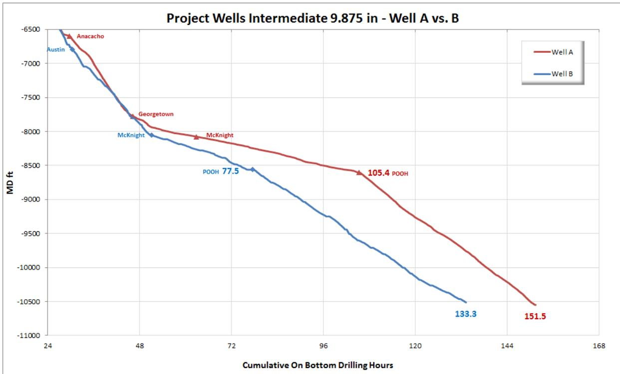
**Figure 22:** Cumulative Drilling Hours vs. Measured Depth – Project Well A vs. B
