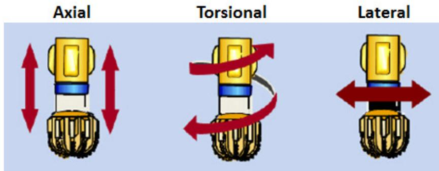
**Figure 5:** Types of Vibrations: Axial, Torsional and Lateral
