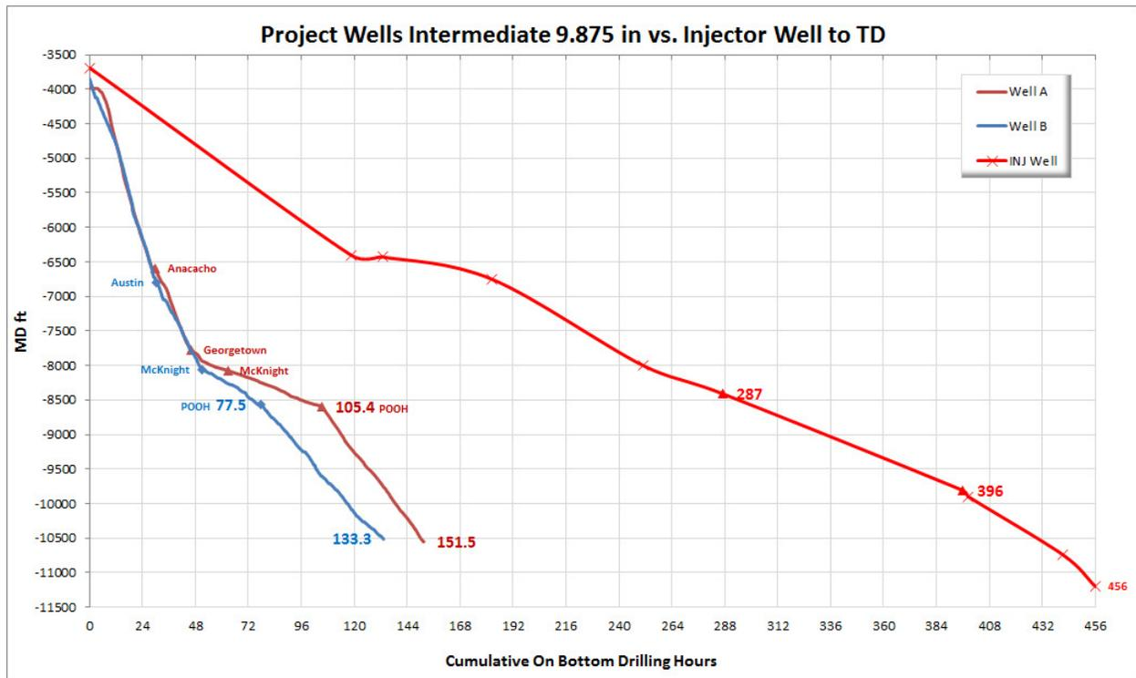
**Figure 23:** Cumulative Drilling Hours vs. Measured Depth – Project Wells A vs. B vs. Injector Well
