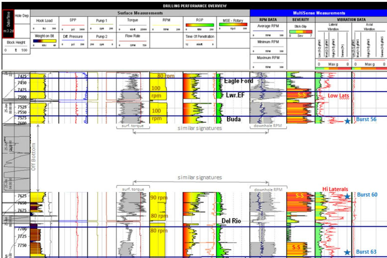
Figure 7: Well A – Stick-Slip Coupled with Lateral Vibrations
