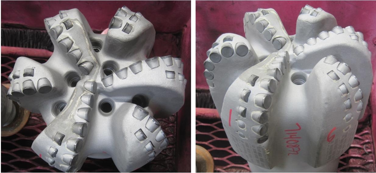
Figure 19: Well B – First 9.875-in PDC Bit with Six Blades and 16mm Cutters
