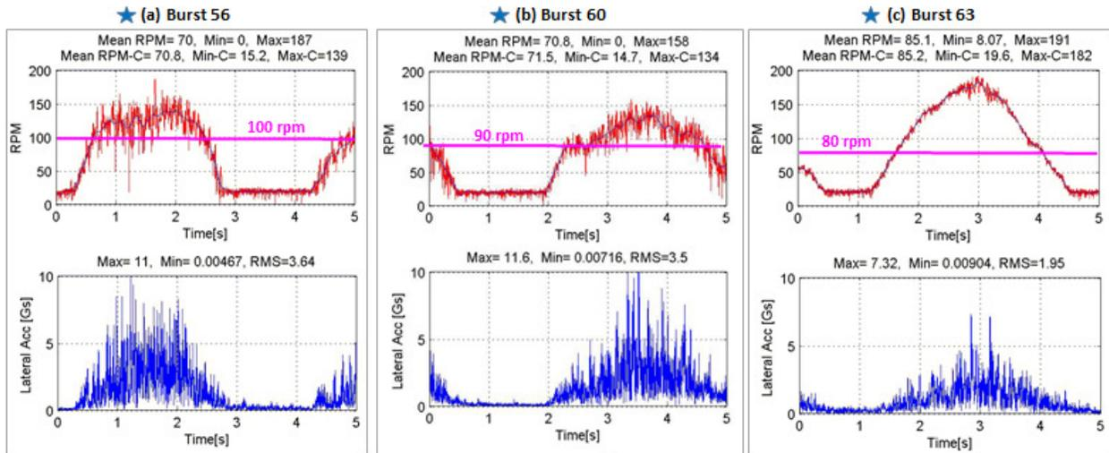
Figure 8: Well A – Burst Plots within Stick-Slip Events
