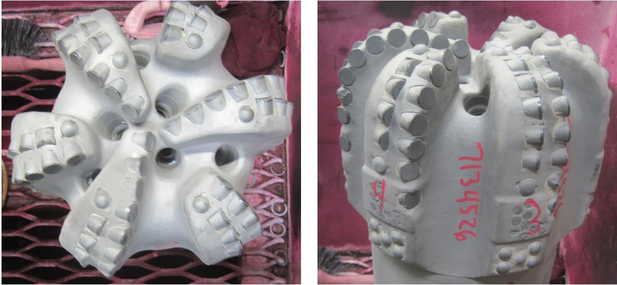
**Figure 21:** Well B – Second 9.875-in PDC Bit with Six Blades and 16mm Cutters
