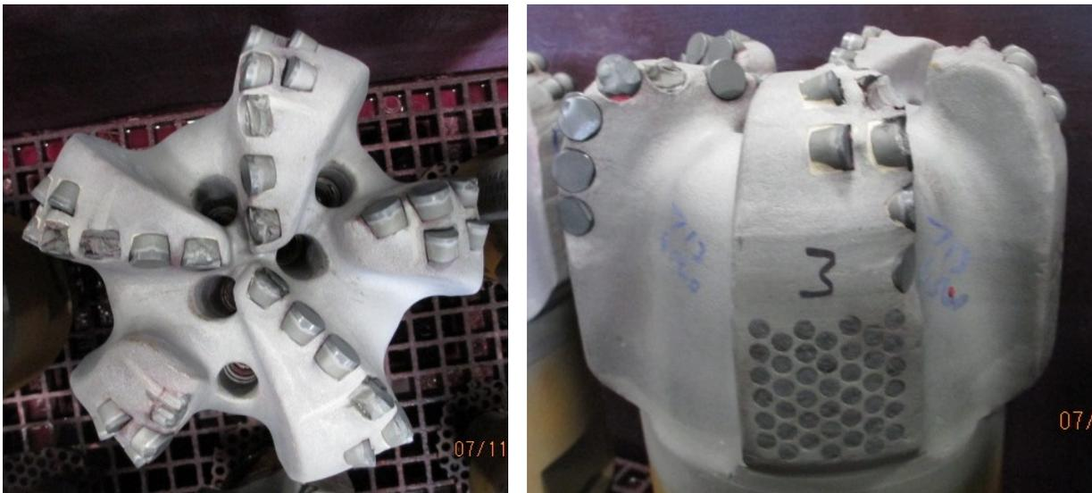
Figure 12: Well A – First 9.875-in PDC Bit with Five Blades and 19mm Cutters
