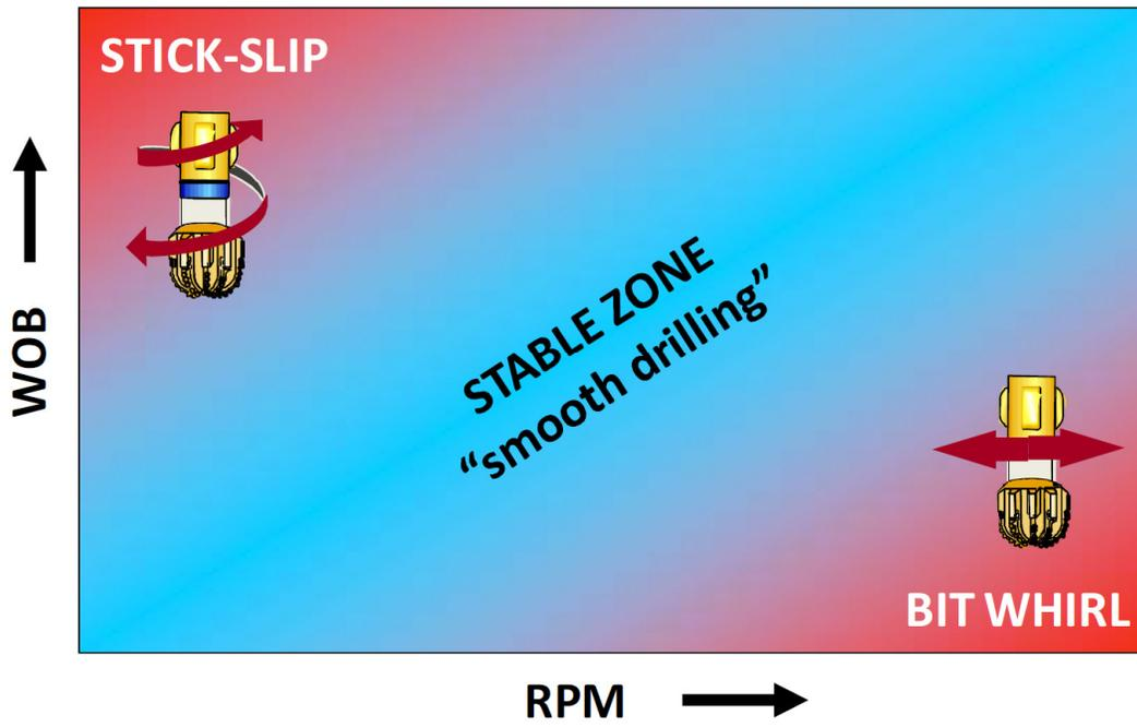
Figure 1: Stability Map of Drilling Dysfunctions for PDC Bits
